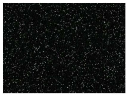
**Figure 2.2** A portion of a frame illuminated by the Fe55 X-ray source with Al foil attenuation.
