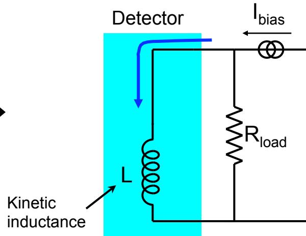
photon absorption disrupts superconductivity locally
