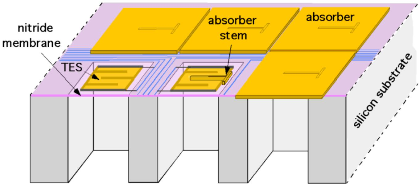
Thick Au/Bi absorber, weak attach
