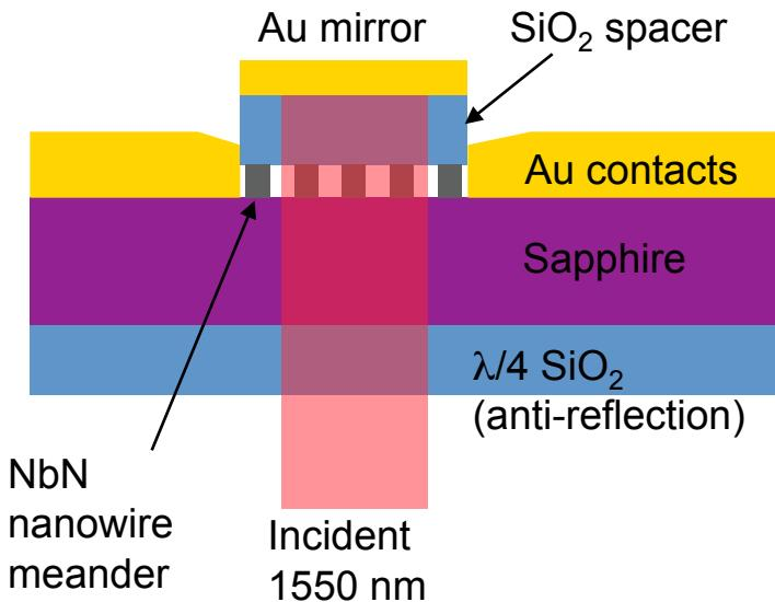
Cavity structure + AR coating
