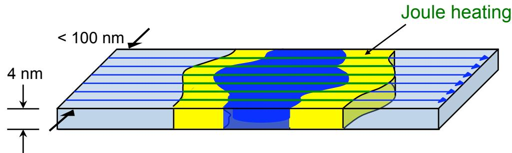
If  $L/R$  is long enough, Joule heating “runs away” ( $R \gg R_{\text{load}}$ ) before current diverted into load
