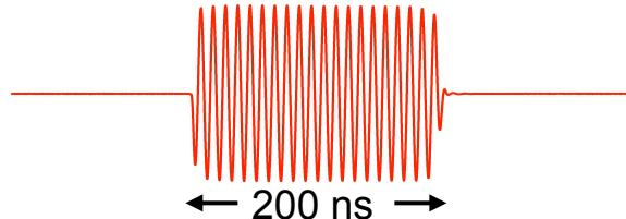
Readout by measuring the reflection coefficient at 1 GHz with low noise cryogenic microwave amplifier
