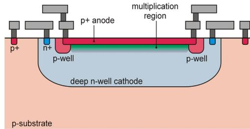
**Fig. 3. Cross-section of the SPAD.**
