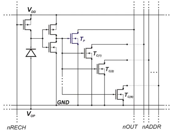
**Fig. 4. Event-driven readout principle: the bus structures.**
