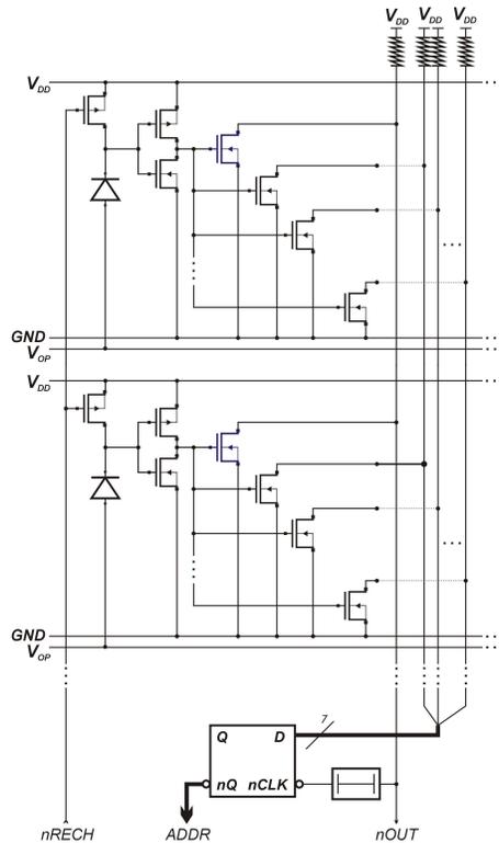
Fig. 5. Complete bus implementation for a single column.
