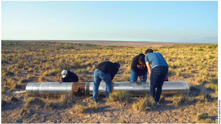
The morning after the launch, the CIBER-2 team recovered the payload, removed the device, extracted the data for analysis, and shipped the device back to Rochester to make modifications in preparation for the next launch.
