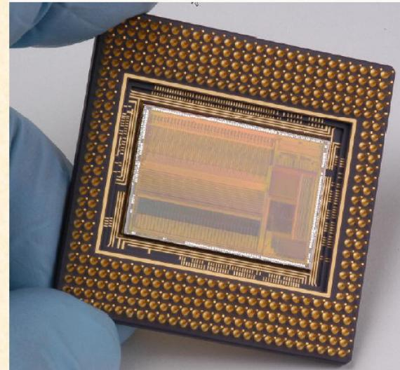
**Figure 2:** Image of the SIDECAR. All signal conditioning, clock/bias generation and digitization hardware is self-contained in this small chip.
