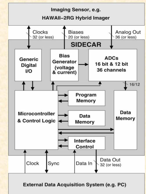
**Figure 5:** Block diagram of the SIDECAR
