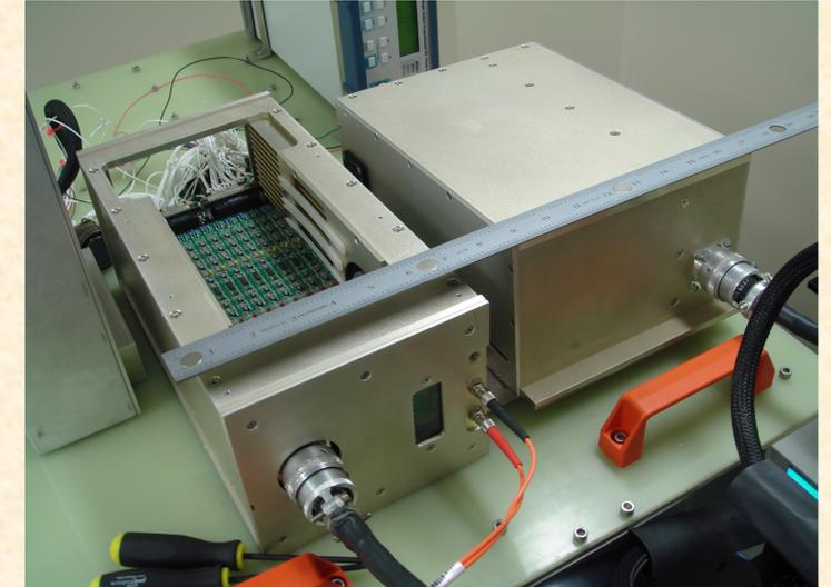
**Figure 3:** Detector control electronics built by Astronomical Research Cameras, Inc. The SIDECAR has the same capability as this set of electronics.
