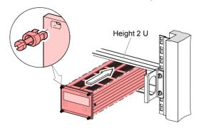
... and fasten the FRG Control Unit to the rack chassis adapter using the screws supplied with it.
