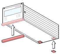
... and slip the supplied rubber bar onto the bottom edge of the front panel.
