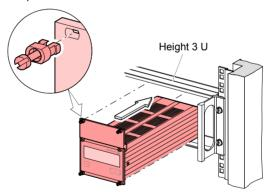
...and fasten the adapter panel to the rack chassis adapter using the screws supplied with the FRG Control Unit.
