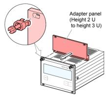
Slide the FRG Control Unit into the rack chassis adapter ...
