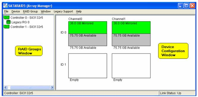
The RAID Groups window identifies SATA host adapters and configured RAID groups. For systems with more than one Silicon Image Host Bus Adapter installed, you can switch between cards by selecting the desired card in the RAID Groups Window.
