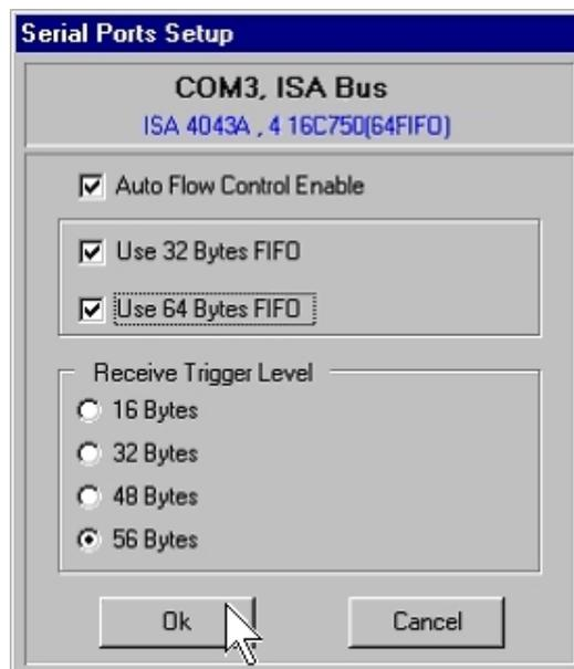
If your card can support 64 (32) bytes FIFO, you can use 16 or 32 or 64 (16 or 32) bytes FIFO. The default value is Use 16 Byte FIFO buffers.
