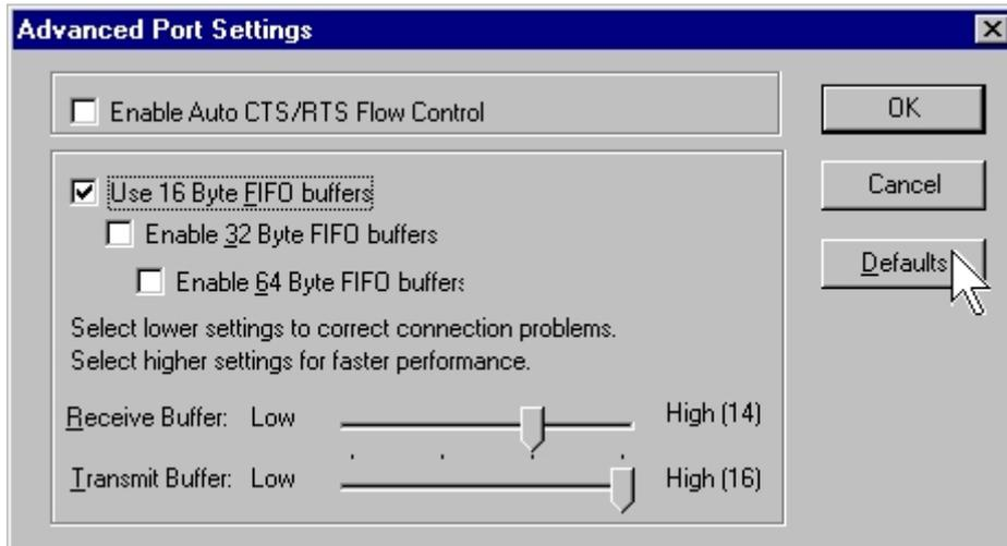
5. Check/un-check the “**Enable CTS/RTS Auto Flow Control**” checkbox to enable/ disable the hardware auto flow control feature.
