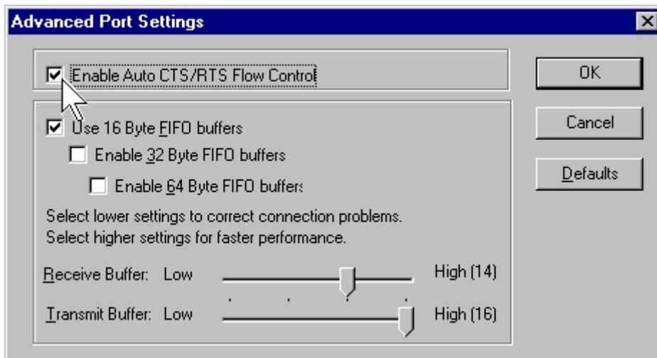
6. Check/Un-check the “**FIFO buffers control**” checkbox to enable / disable the different hardware FIFO buffering features, and you can select the accurate **Receive/Transmit buffer** size of FIFO in control bar.
