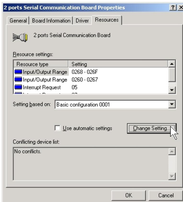
7. Select an available and correct “**Value**” (It depends on the hardware jumper setting.) including IO and IRQ settings and click “**OK**”.
