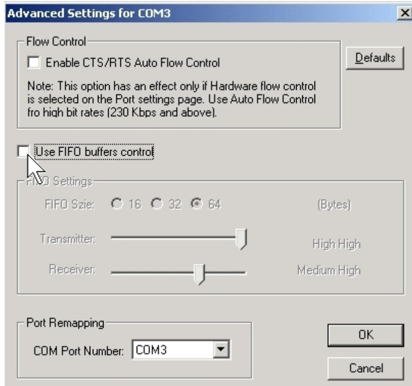
7. Re-map the COM port number by select a free COM port number from the “**COM Port Number**” combo box. The (in use) means this COM port number is used by another COM port.
