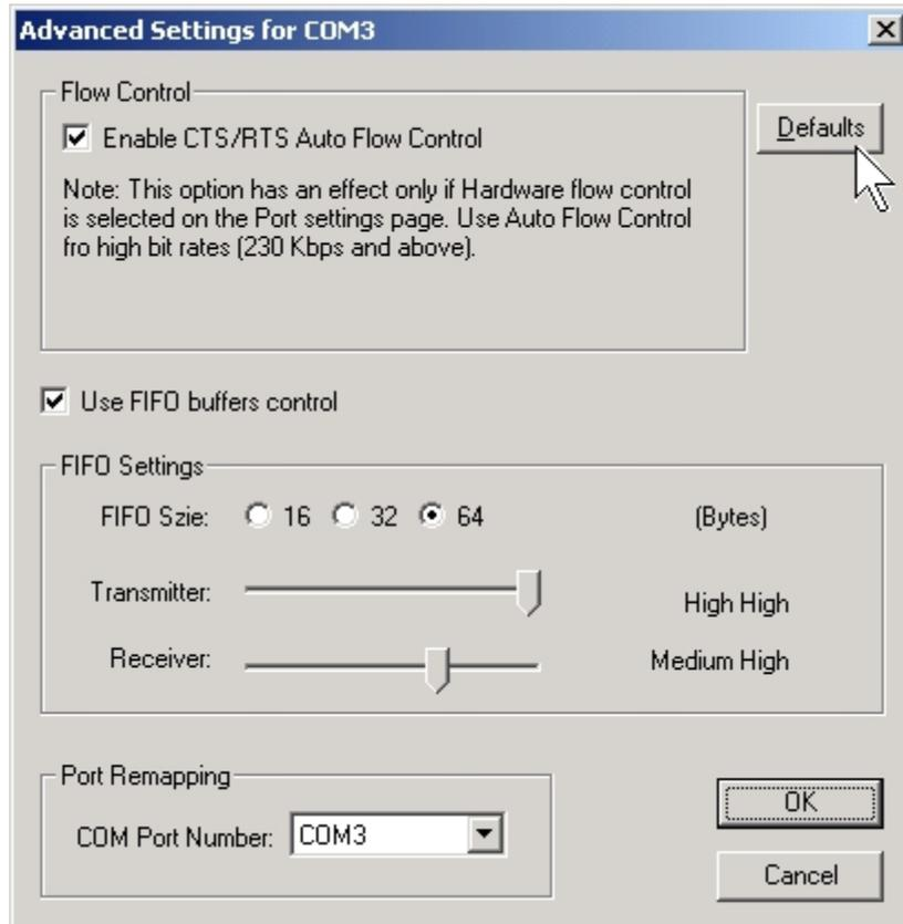
5. Check/un-check the **“Enable CTS/RTS Auto Flow Control”** checkbox to enable/ disable the hardware auto flow control feature.
