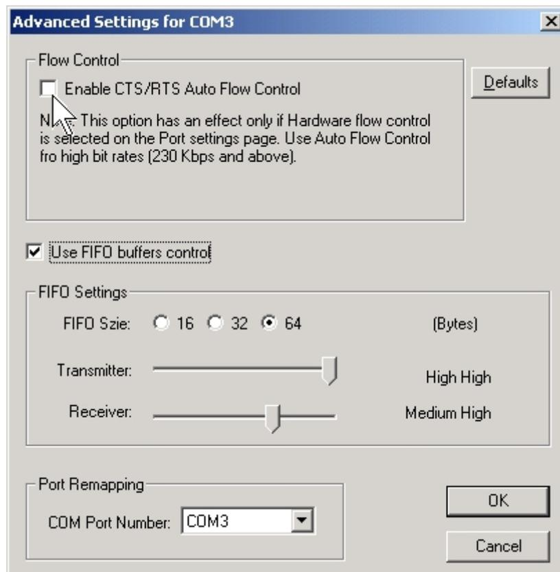
6. Check/Un-check the “**Use FIFO buffers control**” checkbox to enable / disable the hardware FIFO buffering feature or you can select the size of FIFO if “Use FIFO buffers control” is enabled.
