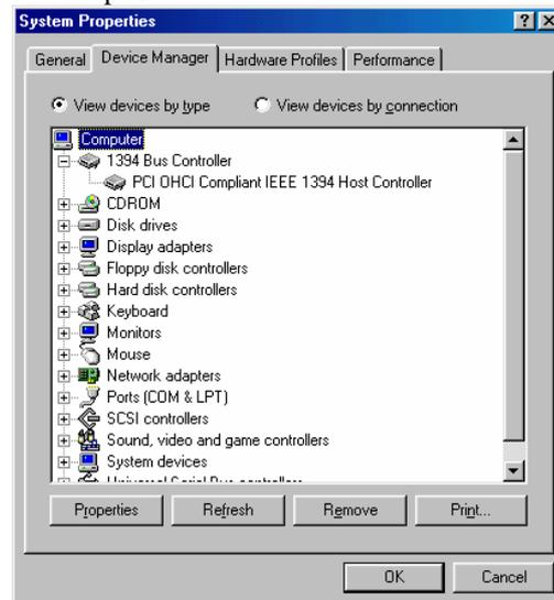
The Windows 98/SE installation CD includes the VIA 1394 OHCI driver, so you do not need an installation CD or diskette. After the installation has finished and the computer has rebooted, you may connect 1394/FireWire devices to it.
