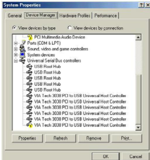
1. Please make sure this PCI card has been installed on your system correctly.
