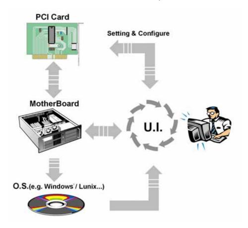
As the flowchart, plug the PCI card on the Motherboard, then install the User Interface software application program under O.S. (e.g. Windows XP). User can control and configure PCI Serial card hardware parameter through this application program..
