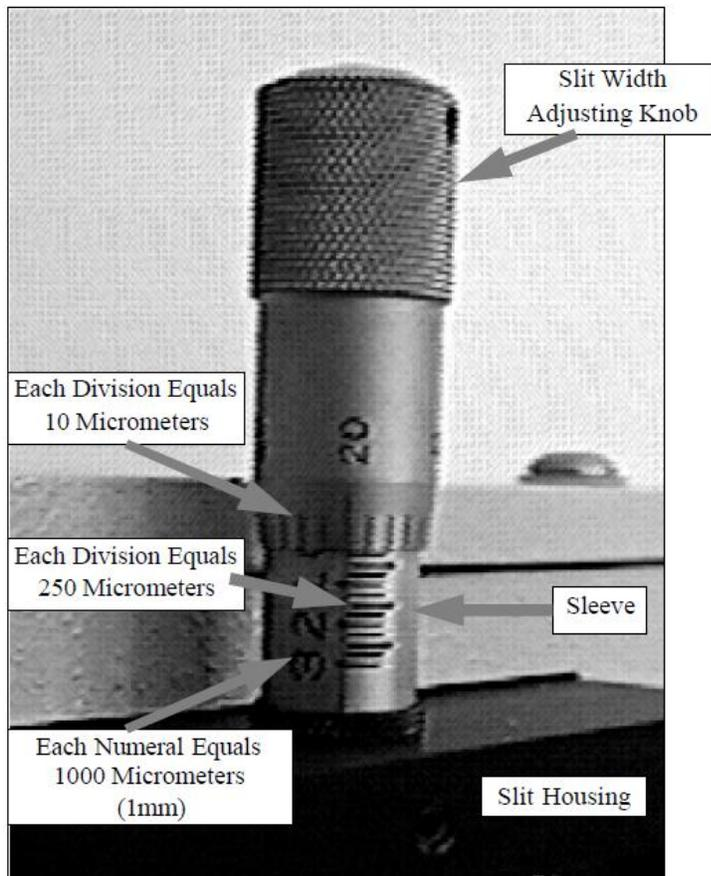
**Figure 7. Slit Width Setting:
