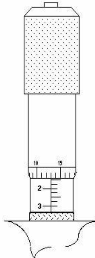
**Figure 8. Slit Width Setting:
