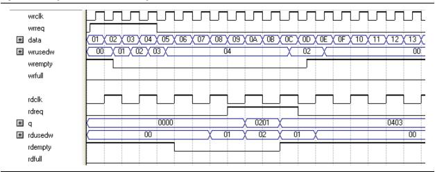
In this example, the read port is operating at half the frequency of the write port. Writing four 8-bit words to the FIFO buffer increases the wrusedw flag to four and the rusedw flag to two. Two 16-bit read operations empty the FIFO. The first and second 8-bit word written are equivalent to the LSB and MSB of the 16-bit output words, respectively. The rdempty signal stays asserted until enough words have been written on the narrow write port to fill an entire word on the wide read port.
