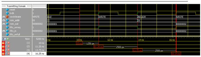
Figure 7. Initial Write Operation to the DCFIFO Megafunction
