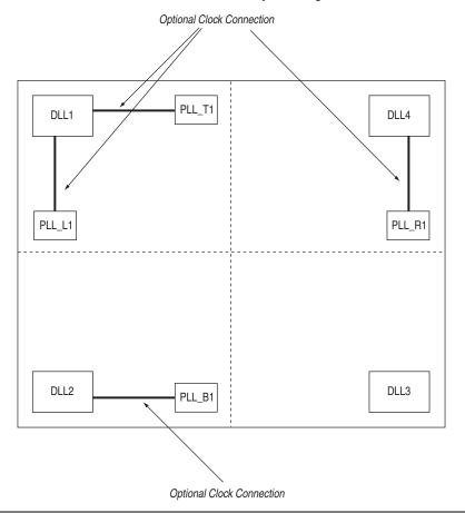
The DLL reference clock should be the same frequency as the memory interface, but the phase is not important.
