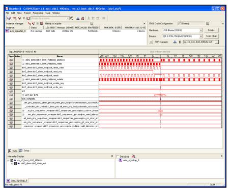
Figure 29. SignalTap II Example DDR2 SDRAM Design Analysis
