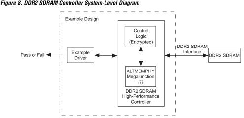
Notes to Figure 8: The ALTMEMPHY megafunction automatically generates the PLL and the PLL is part of the ALTMEMPHY (1)megafunction.
