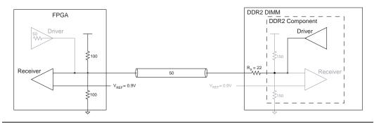
Figure 25. Read Operation From DDR2 SDRAM Using the Parallel OCT Feature of the Stratix III FPGA Device
