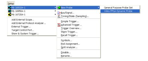
Or, in the Overview window, from a module's drop-down menu, choose New Probe>Xilinx FPGA Dynamic Probe.
