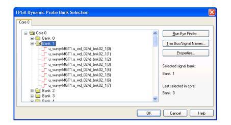
You can correlate internal FPGA activity with external measurements. With each new selection of a signal bank, the application updates new signal names from your design to the logic analyzer. View internal FPGA activity and time correlate internal FPGA measurements with external events in the surrounding system.
