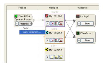
Whenever buses/signals are added to the "FPGA Probe" folder, they are associated with a specific bank. If you select another bank, the added buses/signals do not appear.
