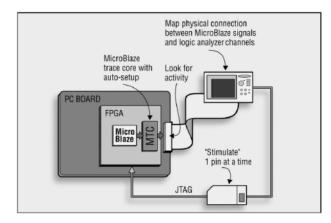
Agilent's MTC reduces the set up time for an initial trace measurement. You can literally connect a logic analyzer to a connector with MTC core outputs routed to it, and within seconds, the logic analyzer becomes ready to take a MicroBlaze trace measurement.
