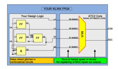
The FPGA dynamic probe will detect the type of ATC2 core and automatically set up the appropriate logic analyzer sampling mode (see page 61).
