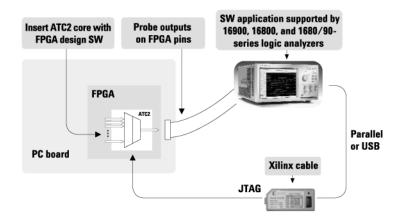
Create a time saving FPGA measurement system. Insert an ATC2 (Agilent Trace Core) core into your FPGA design. With the application running on your logic analyzer via JTAG you control which group of internal signals to measure.
