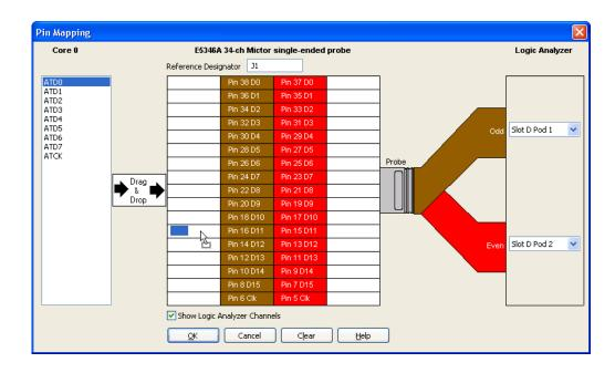
After you've mapped FPGA pins to the probe, you can hover the mouse pointer over a pin description field to view a tool tip describing the FPGA debug pin name, the pod connection, the channel number, and the signal type (single-ended or differential).
