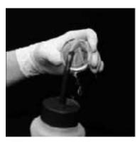
Figure 1. Flushing the optic with Vertrel XF or Asahiklin AK-225.
