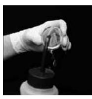
Figure 1. Flushing the optical device with Vertrel XF or Asahiklin AK-225.
