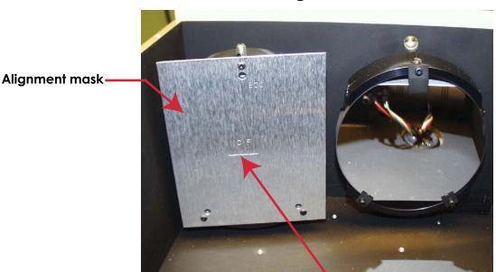
\_Align laser on this short vertical line and horizontal line.
