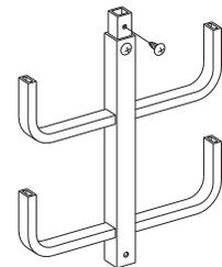
Note: Not to exceed 100 lbs/ft on 12 ft span, 225 lbs/ft on 8 ft span.
