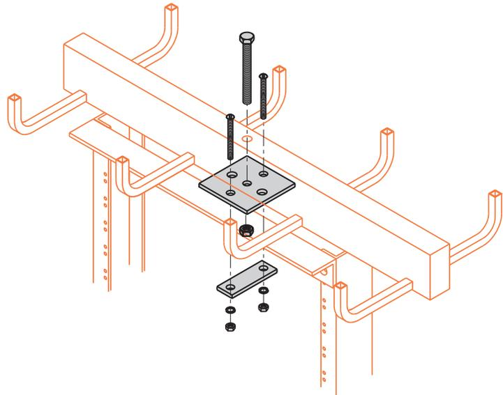
Note: All connectors are aluminum material and sized for 1/2" zinc plated steel hardware, unless otherwise specified.
