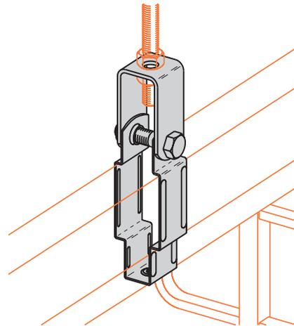
Note: All connectors are aluminum material and sized for 1/2" zinc plated steel hardware, unless otherwise specified.
