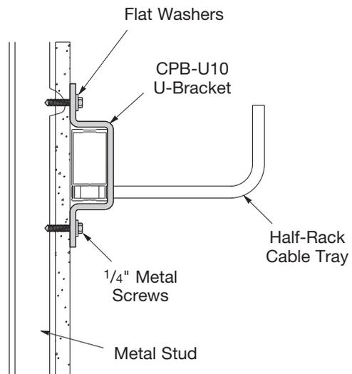
**Note:** These mounting details serve as a vertical support, and can serve as seismic bracing. See the Cent-R-Rail Seismic Restraints brochure for details.
