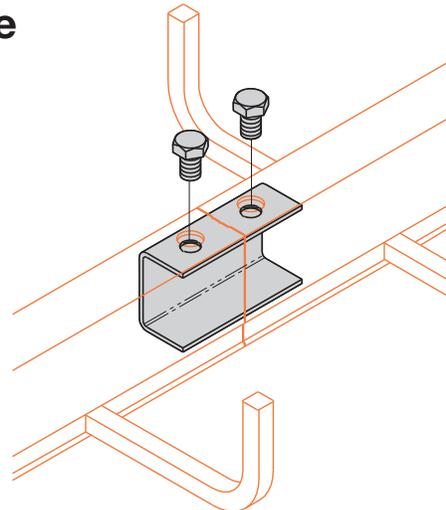
Note: All connectors are aluminum material and sized for 1/2" zinc plated steel hardware, unless otherwise specified.
