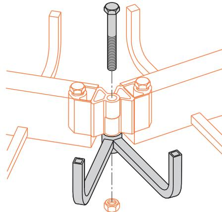
Note: All connectors are aluminum material and sized for 1/2" zinc plated steel hardware, unless otherwise specified.
