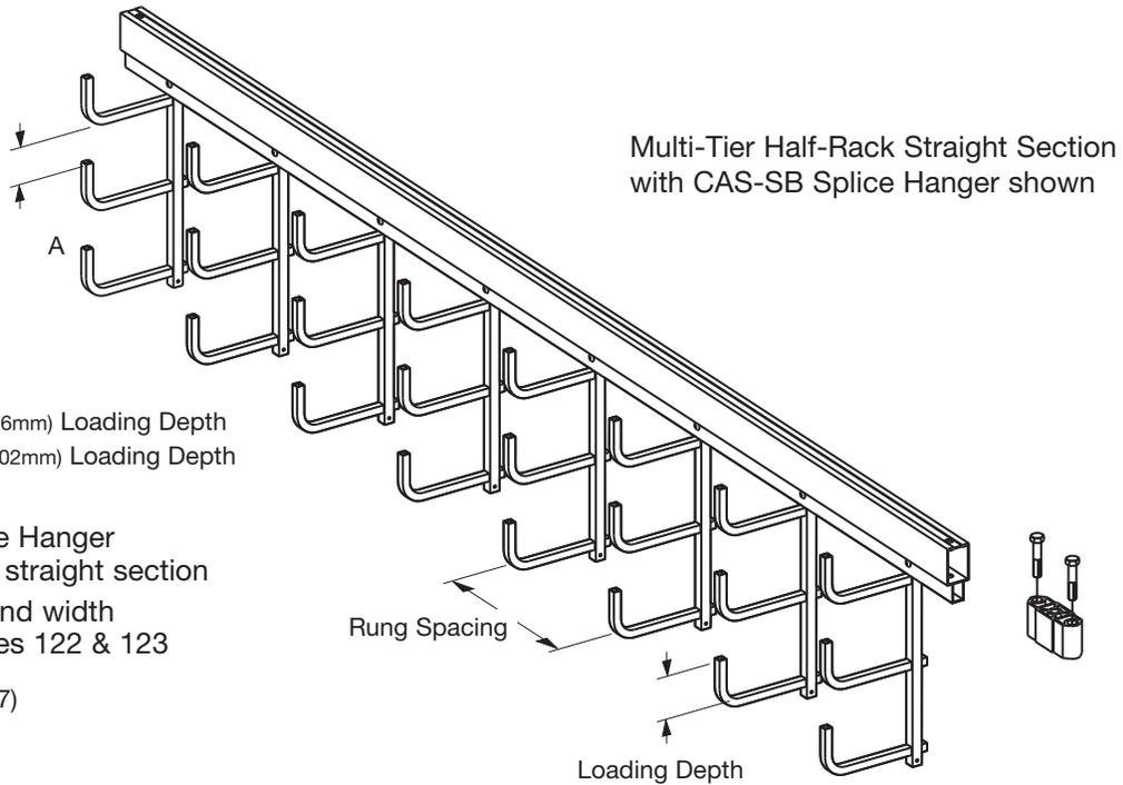
A = 2<sup>5</sup>/<sub>8</sub>" (67mm) for 3" (76mm) Loading Depth
