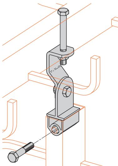
Note: All connectors are aluminum material and sized for 1/2" zinc plated steel hardware, unless otherwise specified.
