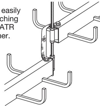
**Note:** Bonding jumper is required to maintain electrical continuity. (pg. 148)
