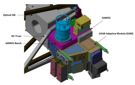
Figure 28. In the rendered image, the SAMOS is mounted to the SOAR Adaptive Module.
