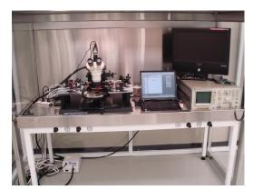
Figure 59. Device wafers are tested in the flow bench lab probe station in the photo above.
