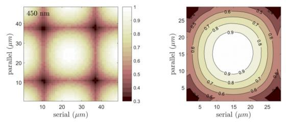
Figure 26. The normalized intrapixel response of Kepler 's CCD at 450 nm, as measured by a spot scanner at RIT, are shown using an intensity map (left) and a contour plot (right). The response is maximal in the central third of a pixel, and rapidly decreases towards the pixel edges.
