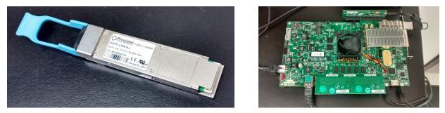
Figure 37. (left) A Xilinx VCU108 FPGA will be used in the EVT station to host various devices, such as a QSFP based package developed by Precision Optical Transceivers (right).
