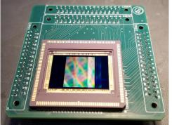
Figure 32. (left) Ben Stewart works on the creation of the cryogenic star tracking attitude regulation system. (right) Shown here is a sCMOS detector mounted to focal plane printed circuit board.
