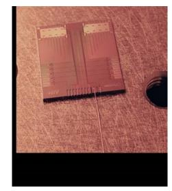
Figure 12. This integrated photonic chip, designed by Precision Optical Transceivers and fabricated by AIM Photonics uses an optical fiber for input and output.
