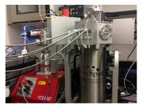
Figure 56. (left) The Integrated Photonics Group acquired space to create the Integrated Photonics Lab to run quantum integrated photonic experiments. (right) Located in the lab is a Photon Spot single photon detector system funded by AFOSR.
