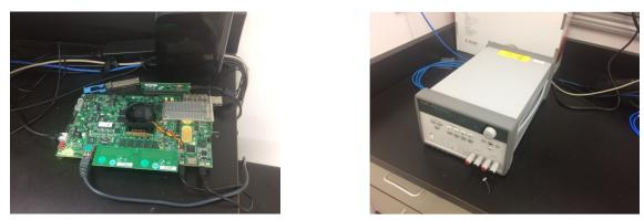
Figure 40. (left) Show in the photo is a VCU108 FPGA board made by Xilinx used in the EVT system. (right) The AgilnetE3649A power supply is being used in testing ProberControl.
