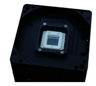
Figure 20. RITPIC uses a CCD and a MOXTEK, Inc. micropolarizer array. Shown above, the micropolarizer array (silver square) is aligned and affixed to the CCD using a white ceramic carrier. The polarizationsensitive imager is inside a camera body, allowing thermoelectric cooling.
