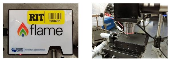
*Figure 58. The electroluminescence measurement setup includes a rotating testing stage (right) and a FLAME 200 nm – 850 nm spectrometer (left).*
