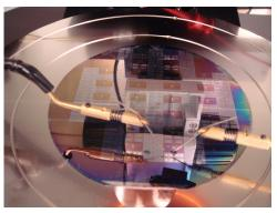
Figure 62. This image is a close-up of a device wafer being tested on the probe station.
