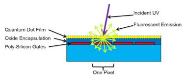
Figure 29. The cross-section schematic shows a quantum dot coated device.
