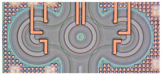
Figure 6. Above is a microscope image of an entangled photon source on an integrated photonic chip.
