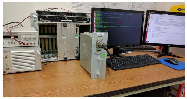
Figure 13. The image shows the benchtop setup used to develop a data acquisition and analysis system for the TIME-Pilot instrument.
