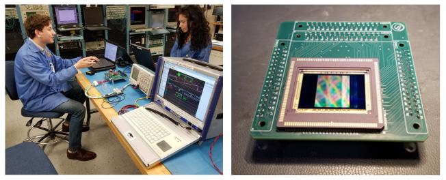
Figure 11. (left) Undergraduate students Ben Stewart and Ambar deStantiago complete telemetry stream interfacing at the NASA Wallops Flight Facility. (right) The project used a 5.5 megapixel sCMOS detector mounted on a custom printed circuit board.
