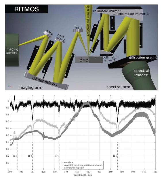
Figure 23. (top) This graphic shows how a DMD splits light into a spectral imaging arm and an imaging arm within the RIT Multi-Object Spectrograph (RITMOS). (bottom) These are spectra of Beta Per, obtained by RITMOS using the new DMD device. Hydrogen absorption lines are marked for better visibility. Y-axis represents normalized intensity and is unitless.
