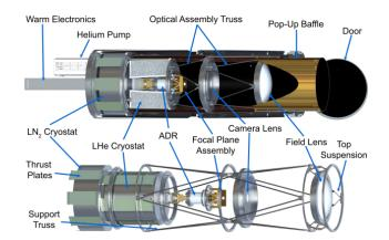
Figure 33. The image above is a mechanical model for a NASA proposed project, the Rocket Axion Decay Experiment (RAxDEx)
