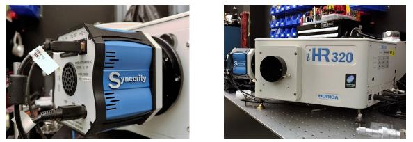
Figure 57. The Syncerity CCD Array detector (left) and the HR320 spectrometer (right) are part of the photoluminescence system.
