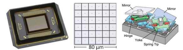
Figure 22. (left) The picture shows a DMD with a custom UV-enhanced sapphire window. (middle) A microscope image shows 36 individual micromirrors. (right) A schematic shows the hinge and tilt mechanism for two micromirrors.
