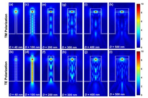
Figure 14. (top) This shows the cross-sectional near-field electric field intensity of nanowire UV LEDs with  $H = 1 \mu m$  and various diameters for TM-polarization (bottom) and TE-polarization.
