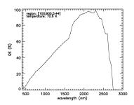
Figure 2. The QE of a thinned part extends below 1.1  $\mu$ m, as expected.
