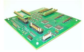
Figure 63. This image shows a cryogenic multi-layer circuit board designed in the CfD and populated in CEMA. All of the components on this board work at temperatures as low as 40 K, nanoTorr pressure levels, and in the presence of high energy particle radiation.
