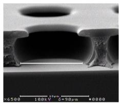
*Figure 60. (left) The Amray 1830 Scanning Electron Microscope is used to image devices. (right) The SEM image shows a sample prepared for indium bump deposition.*
