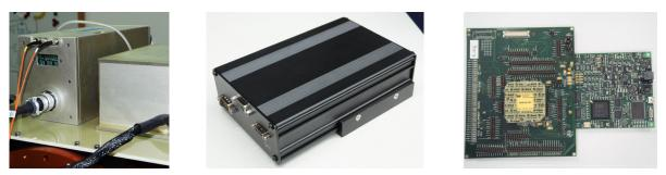
Figure 52. The three electronics packages used to test detectors are the Astronomical Research Camera Controller (left), JMClarke Engineering (middle), and the Teledyne SIDECAR ASIC (right).
