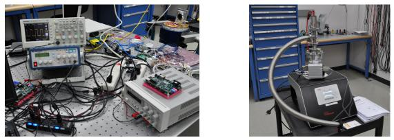
Figure 64. (left) Pictured here are the function generators, oscilloscopes, and FPGA-based control boards used to develop an image sensor readout package that will fly on a suborbital platform. (right) The picture shows one of the Oerlikon Leybold Turbolab turbo-molecular pumping stations in the lab.
