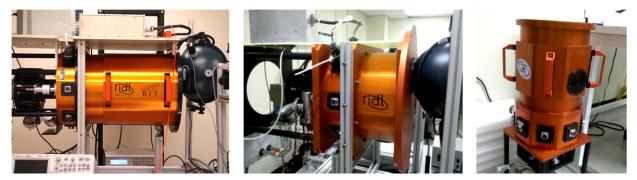
Figure 53. Detectors are evaluated in four custom dewar test systems. The fourth dewar (not pictured) is a duplicate of the one on the left.
