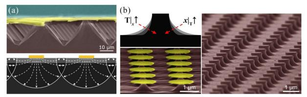
Figure 35. (left) This image shows the fabrication of suspended III-V nanofoils by inverse metal-assisted chemical etching of In<sub>0.49</sub>Ga<sub>0.51</sub>P/GaAs heteroepitaxial films, and (middle) ordered Al<sub>x</sub>Ga<sub>1-x</sub>As nanopillar arrays via inverse metal-assisted chemical etching.
