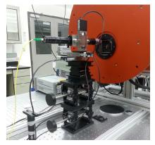
Figure 54. A laser spot projector with three-axis motion control system is used to project a small spot of light within individual pixels of detectors in order to measure the response in all regions of a pixel.
