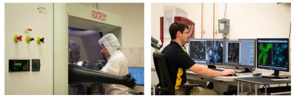
Figure 65. (left) PhD student Mohad Baboli loads a sample in the AIXTRON 3×2 Close Coupled Showerhead metal-organic chemical vapor deposition reactor, part of the MOVPE. (right) PhD student Thomas Wilhelm uses a TESCAN MIRA3 scanning electron microscope to analyze samples for use in metal-assisted chemical etching experiments.
