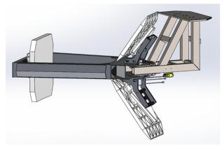
Figure 36. Shown above is a current model of the k-mirror project.
