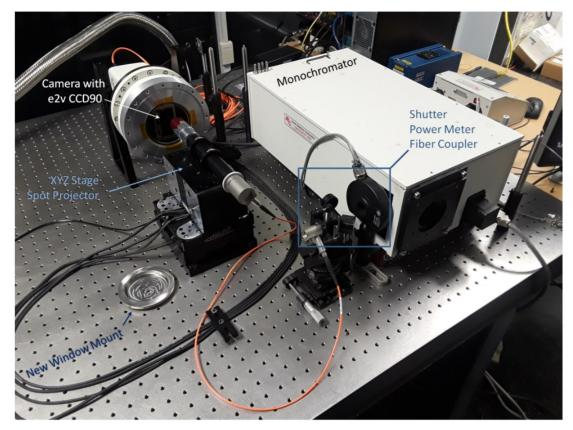
Figure 25. A new apparatus to measure the intrapixel response function of a range of imaging arrays was built in RIT's Laboratory for Advanced Instrumentation Research. This system produces small spots of light across a wide range of wavelengths.
