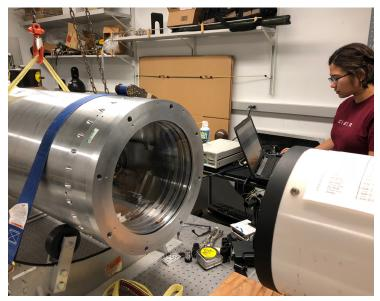
Figure 18. Chi Nguyen takes test images to characterize the CIBER-2 telescope as the payload is being cooled to 77 K.
