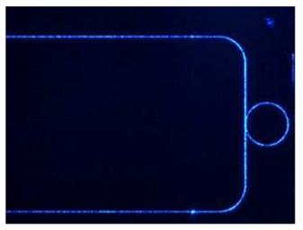
Figure 5. The image shows visible light propagating in an aluminum nitride waveguide and ring resonator.
