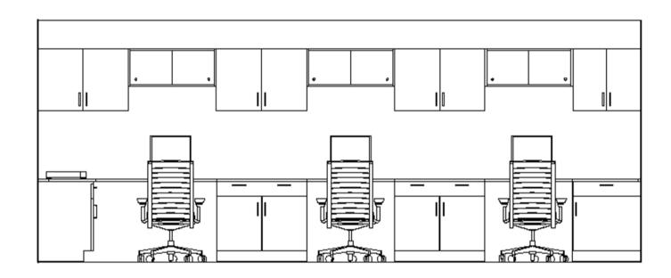
Workstations in the lab with upper and lower cabinet storage – sliding glass panels above
