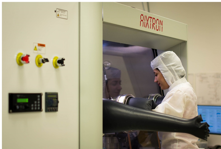
Figure 21. Mohad is seen here loading a sample in the AIXTRON 3×2 Close Coupled Showerhead metal-organic chemical vapor deposition (MOCVD; RIT NanoPower Research Laboratories) reactor for crystal growth of III-V semiconductor nanowires.
