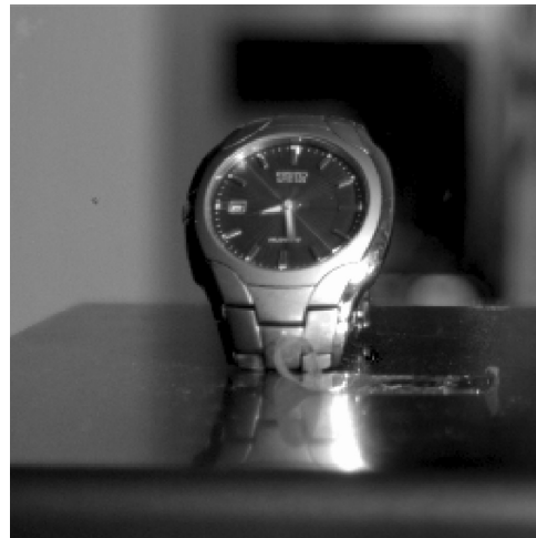
Figure 14. The photos show images of a watch taken with the GM-APD detector arrays developed in this project. The improvement in the image is due to the use of a better bonding process.
