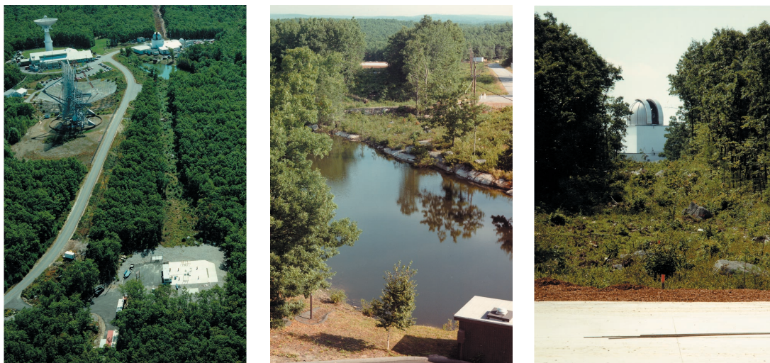
FIGURE 15. Photographs of the 500-m propagation range at the Lincoln Laboratory Firepond facility in Westford, Massachusetts. On the left is an aerial view with the Firepond dome at top right and the target pad at bottom right. The middle image shows the view from the dome toward the target pad, and the right image shows the view from the pad to the dome. The 3D-ladar brassboard, low-light-level intensity camera, and diode laser were housed within a few inches of one another in the dome. At nighttime, the diode laser illuminated the scene for the camera.
