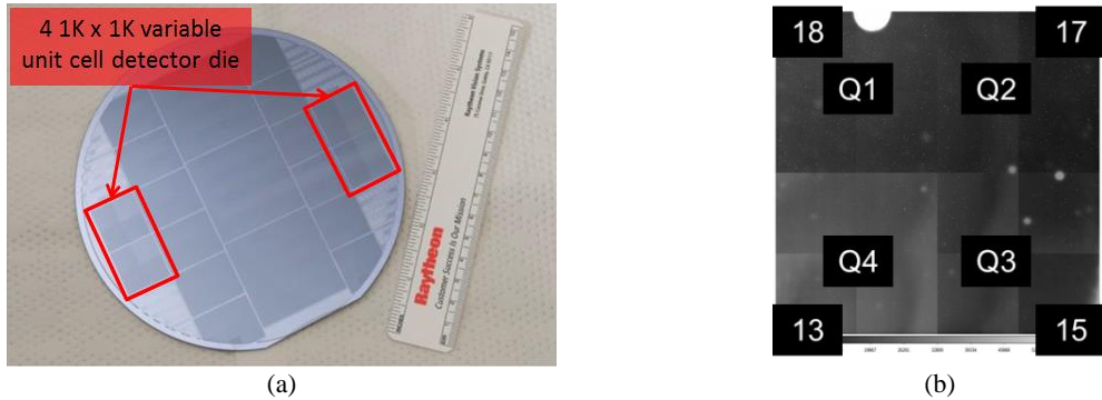
Figure 3. (a) The image shows a wafer that has 2K and 1K die, including 1K versions that have VUC designs. (b) The picture shows a dark image taken with one of the VUC devices with the mesa size ( \mu\text{m} ).
