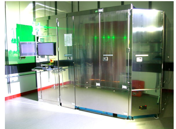
EBL tool: Jeol 8100FS – 200 mm (only 3 in N. America)
