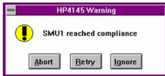
Figure 15: ICS Reports Compliance Events if the Report Compliance Switch is Selected in the Mainframe Setup Dialogue Box.
