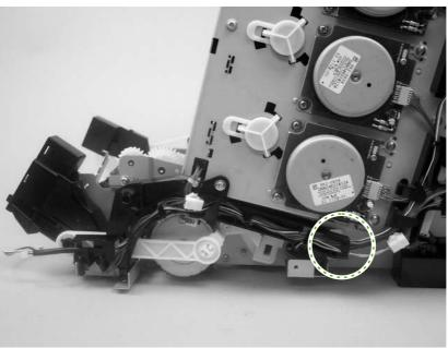
**8.** Release the retainer tabs on the ETB connector link arm (callout 11) and slide the link arm off of the pivot pin.
