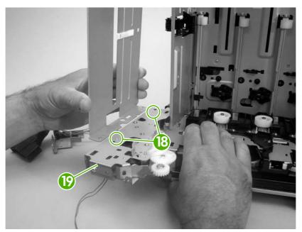
Figure 5-69 Remove the pickup-drive assembly (12 of 13)
