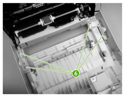
Figure 5-9 Remove the front cover (6 of 7)
