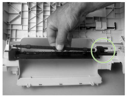
Figure 5-36 Remove the duplex-reverse-drive assembly (2 of 5)
