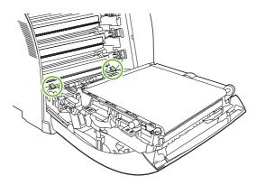
**6.** Press the tabs, and then lift the registration plate. Remove any jammed media, and then return the registration plate to its closed position.
