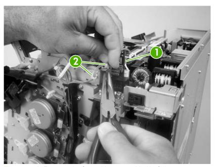
Figure 5-42 Remove the fuser drive assembly (1 of 4)
