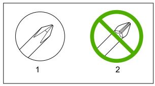
Figure 5-1 Phillips and pozidrive screwdriver comparison
