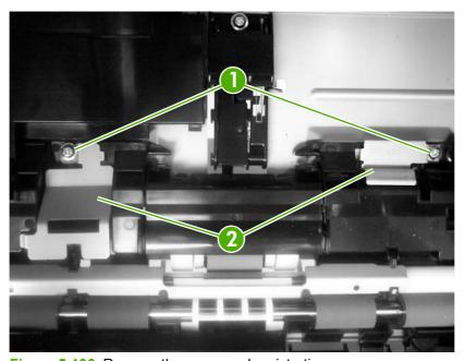
Figure 5-106 Remove the paper and registration sensor covers
