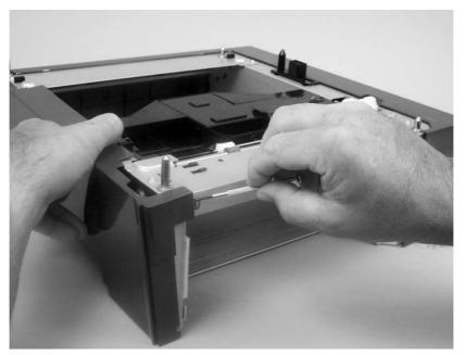
Figure 5-116 Remove the 500-sheet feeder left cover (3 of 5)
