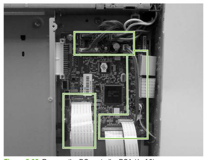
Figure 5-85 Remove the DC controller PCA (1 of 3)
