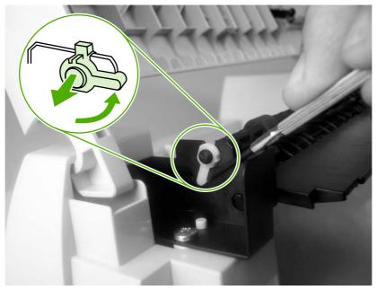
Figure 5-35 Remove the duplex-reverse-drive assembly (1 of 5)
