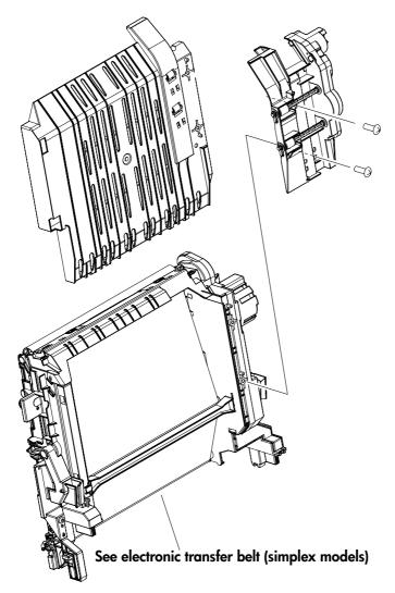
Figure 7-19 Electronic transfer belt (duplex models)
