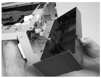
Figure 5-113 Remove the 500-sheet feeder right cover (3 of 3)
