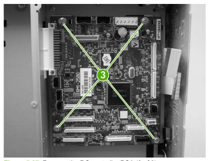
Figure 5-87 Remove the DC controller PCA (3 of 3)
