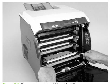
Figure 5-3 Remove the print cartridges (2 of 2)
