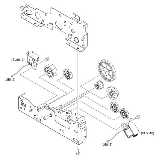
Figure 7-10 Paper-pickup drive assembly
