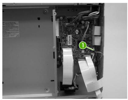
Figure 5-77 Remove the main fan (1 of 2)
