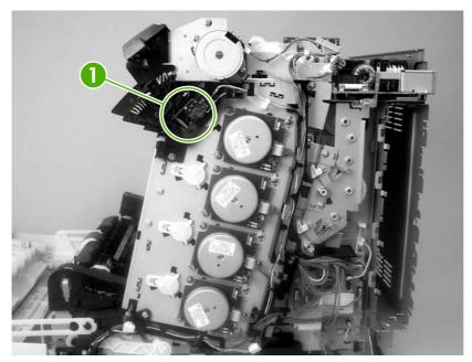
Figure 6-3 Door switch and fuser interlock
