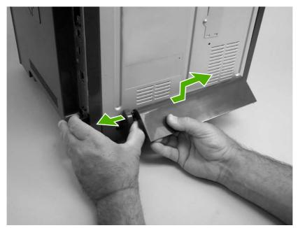
Figure 5-16 Remove the rear lower cover (1 of 2)
