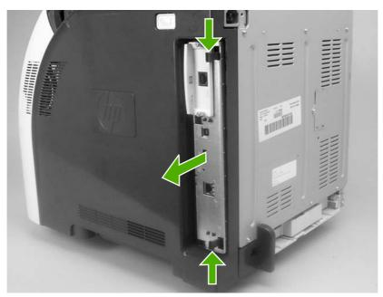
Figure 5-28 Remove the formatter cage
