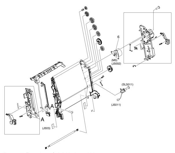
Figure 7-18 Electronic transfer belt (simplex models)
