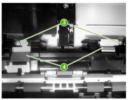
Figure 5-52 Remove the pickup-and-feed assembly (3 of 8)
