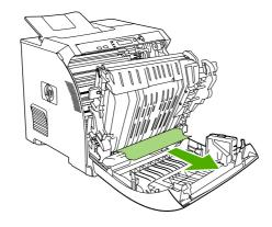
5. Locate the green registration-plate tabs that are below the bottom print cartridge.
