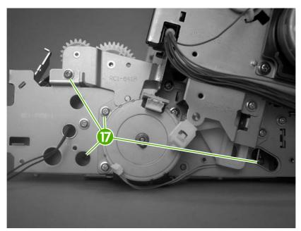
Figure 5-68 Remove the pickup-drive assembly (11 of 13)
