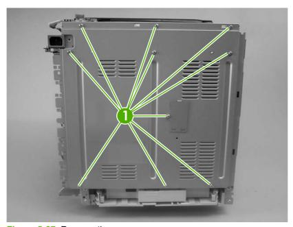
Figure 5-27 Remove the rear upper cover
