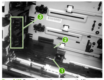
Figure 5-103 Remove the cassette media sensor (1 of 2)
