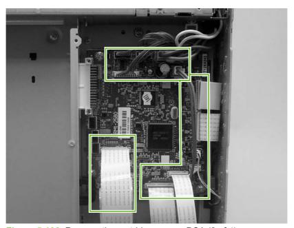
Figure 5-108 Remove the cartridge-sensor PCA (2 of 4)
