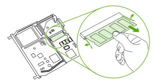
**4.** Remove the new DIMM from the antistatic package, and then locate the alignment notch on the bottom edge of the DIMM.
