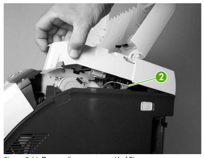
Figure 5-14 Remove the upper cover (4 of 5)
