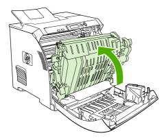
4. Remove any jammed sheets from under the transfer unit.
