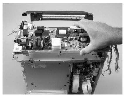
Figure 5-84 Remove the low-voltage power-supply PCA (6 of 6)
