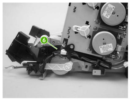
Figure 5-61 Remove the pickup-drive assembly (4 of 13)
