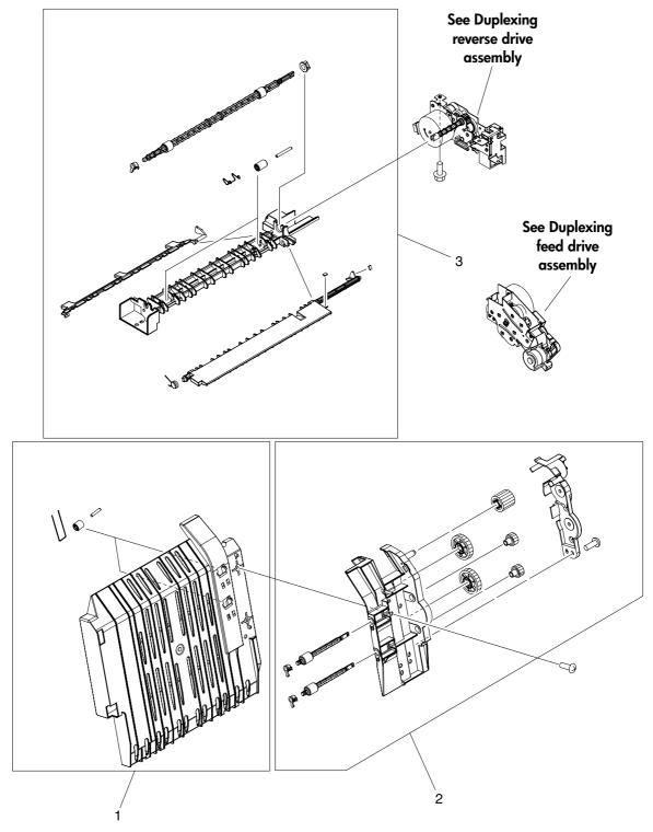
Figure 7-21 Duplex-paper feed assembly (duplex models)
