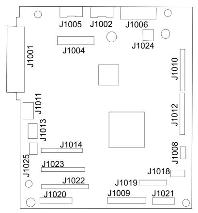
Figure 6-12 DC controller connectors
