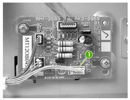
Figure 5-124 Remove the media sensor (500-sheet feeder) (1 of 4)
