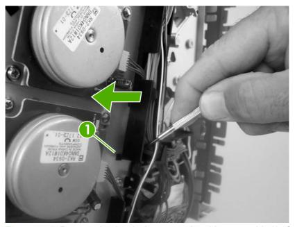
Figure 5-46 Remove the developing separation-drive assembly (1 of 4)
