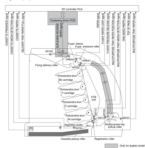
Figure 4-6 Pickup-and-feed system sensors
