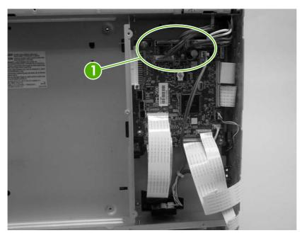
Figure 5-79 Remove the low-voltage power-supply PCA (1 of 6)
