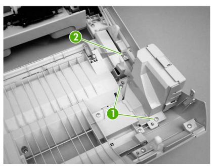
Figure 5-31 Remove the duplex fan (1 of 3)
