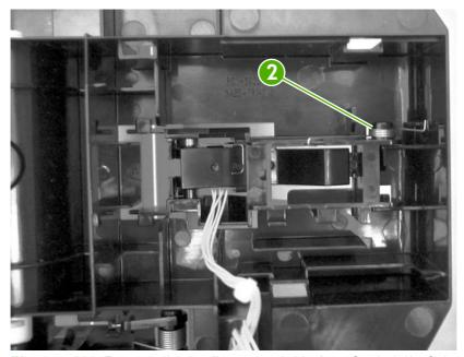
Figure 5-126 Remove the media sensor (500-sheet feeder) (3 of 4)
