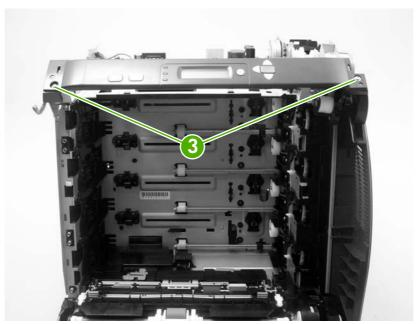
Figure 5-96 Remove the control panel (2 of 2)
