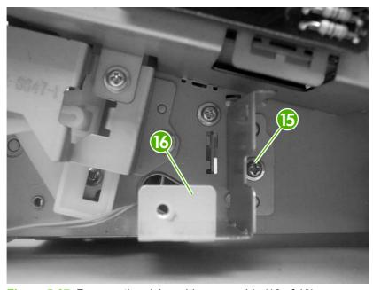
Figure 5-67 Remove the pickup-drive assembly (10 of 13)
