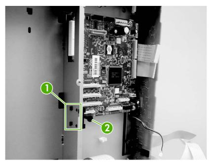
Figure 5-86 Remove the DC controller PCA (2 of 3)
