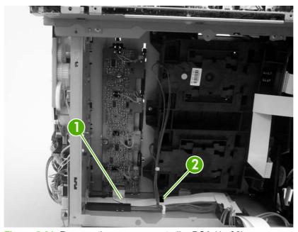
Figure 5-91 Remove the memory-controller PCA (1 of 2)
