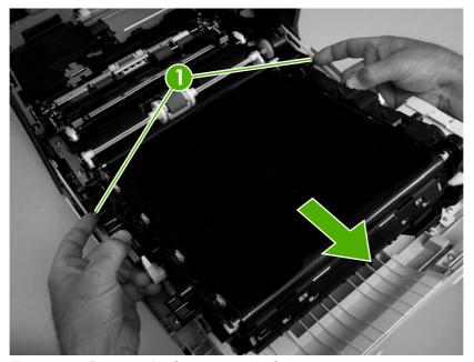
Figure 5-4 Remove the front cover (1 of 7)
