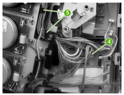
Figure 5-44 Remove the fuser drive assembly (3 of 4)
