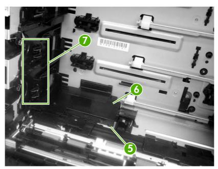
Figure 5-53 Remove the pickup-and-feed assembly (4 of 8)
