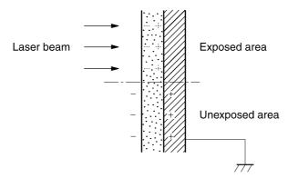
Figure 4-12 Laser-beam exposure
