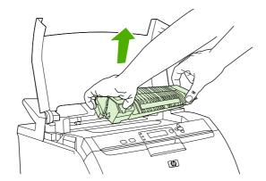
**5.** On the fuser, lift the shutter door.
