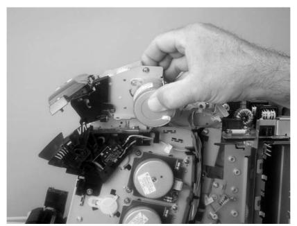
Figure 5-41 Remove the duplex-feed-drive assembly (2 of 2)
