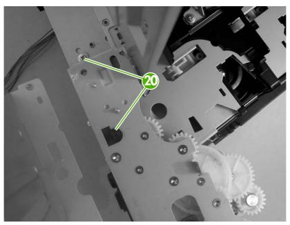
Figure 5-70 Remove the pickup-drive assembly (13 of 13)
