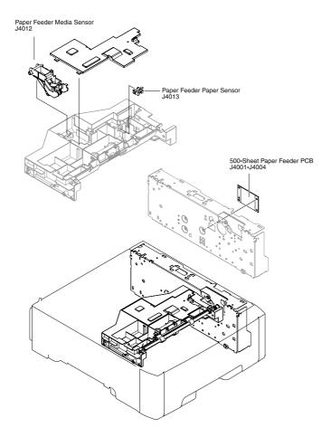
Figure 6-6 500-sheet tray connector locations
