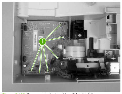
Figure 5-100 Remove the duplex-driver PCA (1 of 3)
