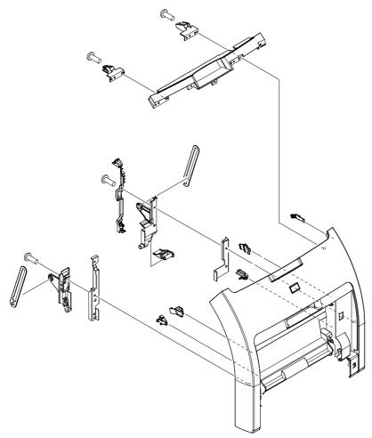
Figure 7-3 Front-cover assembly (simplex model)
