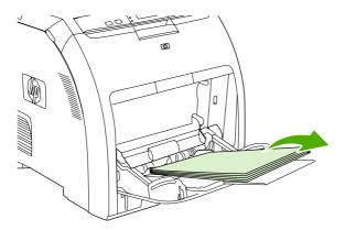
2. Grasp the jammed sheet by both corners and pull.
