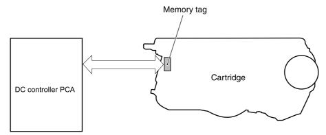
Figure 4-18 Print-cartridge activation
