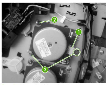
Figure 5-34 Remove the print-cartridge motor
