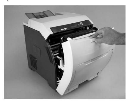
**CAUTION** Do not place any item on the transfer unit while it is open. If the transfer unit is punctured, print-quality problems could result.
