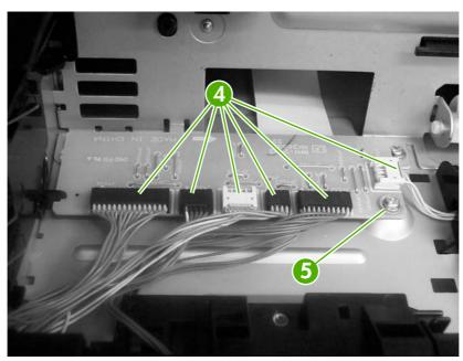
Figure 5-99 Remove the pickup-and-feed driver PCA (3 of 3)
