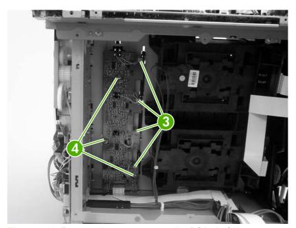
Figure 5-92 Remove the memory-controller PCA (2 of 2)
