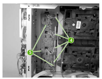
Figure 5-110 Remove the cartridge-sensor PCA (4 of 4)
