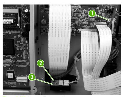
Figure 5-105 Remove the temperature sensor
