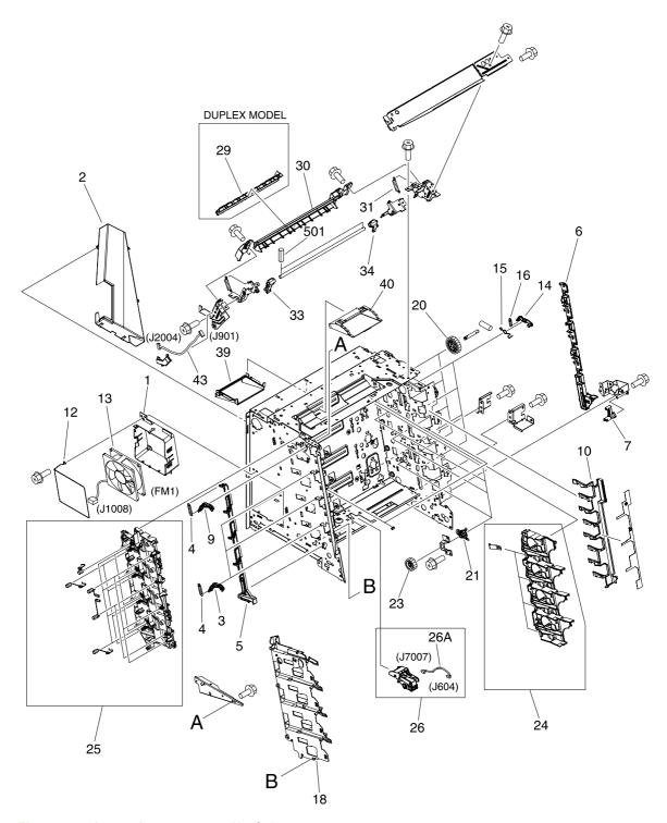
Figure 7-5 Internal components (1 of 5)
