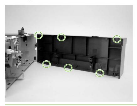
2. Carefully pry loose the two locking tabs along the top of the cover.
