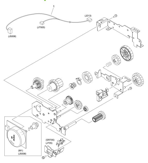
Figure 7-14 Fuser drive assembly
