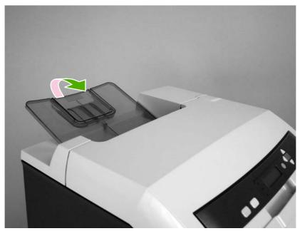
Figure 5-11 Remove the upper cover (1 of 5)
