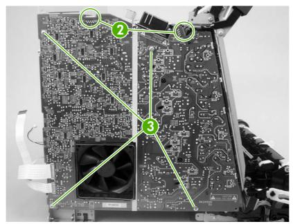
Figure 5-89 Remove the high-voltage power supply (2 of 3)
