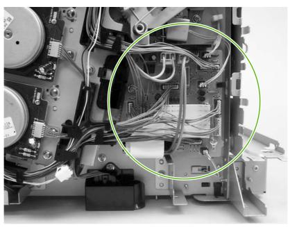
Figure 5-93 Remove the driver PCA (1 of 2)
