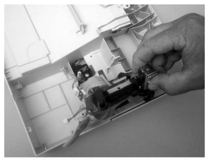
Figure 5-39 Remove the duplex-reverse-drive assembly (5 of 5)
