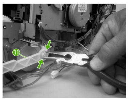
Figure 5-64 Remove the pickup-drive assembly (7 of 13)
