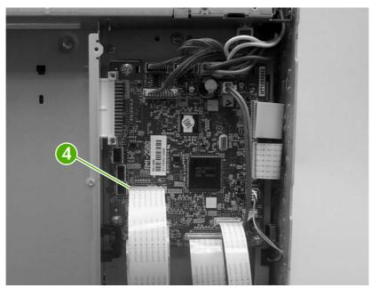
Figure 5-98 Remove the pickup-and-feed driver PCA (2 of 3)
