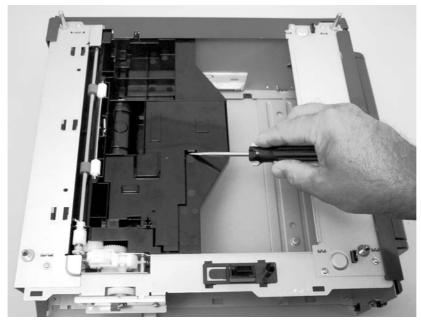
Figure 5-125 Remove the media sensor (500-sheet feeder) (2 of 4)
