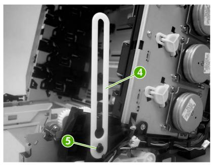
Figure 5-60 Remove the pickup-drive assembly (3 of 13)
