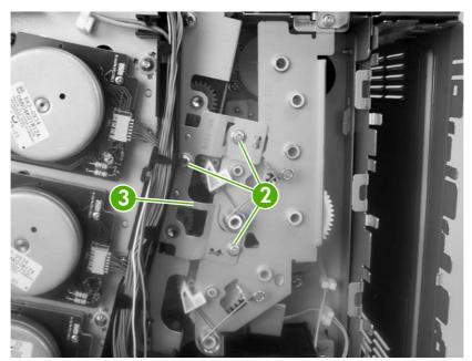
Figure 5-47 Remove the developing separation-drive assembly (2 of 4)
