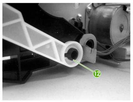
Figure 5-65 Remove the pickup-drive assembly (8 of 13)
