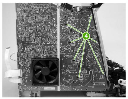
Figure 5-90 Remove the high-voltage power supply (3 of 3)
