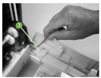
Figure 5-32 Remove the duplex fan (2 of 3)
