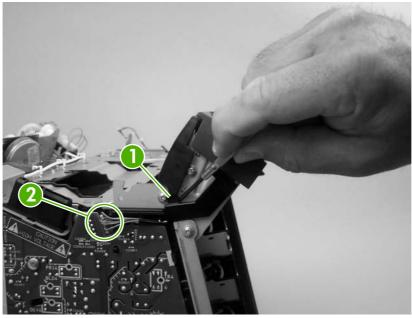
Figure 5-95 Remove the control panel (1 of 2)
