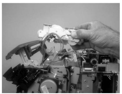
Figure 5-45 Remove the fuser drive assembly (4 of 4)
