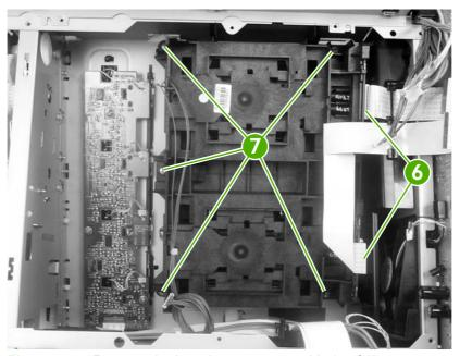
Figure 5-75 Remove the laser/scanner assembly (5 of 6)
