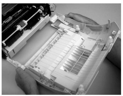
Figure 5-10 Remove the front cover (7 of 7)
