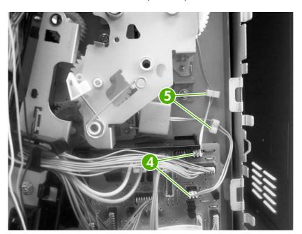
Figure 5-48 Remove the developing separation-drive assembly (3 of 4)
