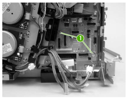
Figure 5-94 Remove the driver PCA (2 of 2)
