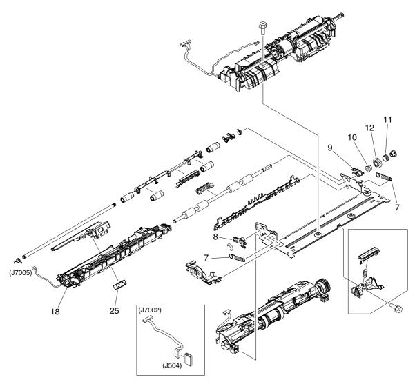
Figure 7-17 Paper-pickup assembly (HP CLJ 3000)
