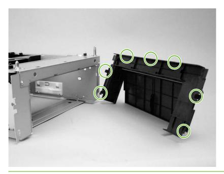
**ENWW** 500-sheet feeder 161 3. Carefully pry loose the three locking tabs along the top of the cover.
