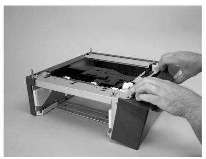
Figure 5-112 Remove the 500-sheet feeder right cover (2 of 3)
