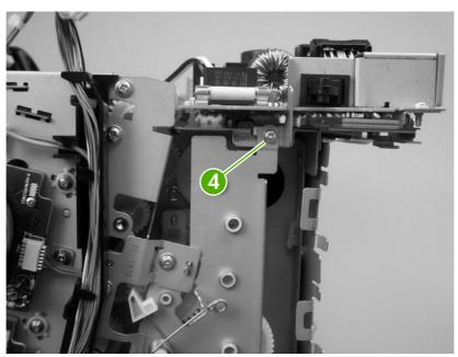
Figure 5-81 Remove the low-voltage power-supply PCA (3 of 6)
