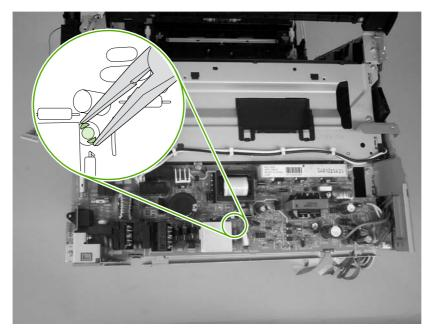
Figure 5-83 Remove the low-voltage power-supply PCA (5 of 6)
