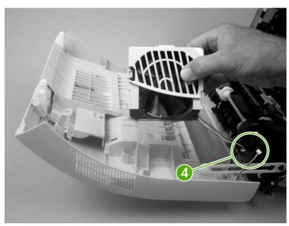
Figure 5-33 Remove the duplex fan (3 of 3)
