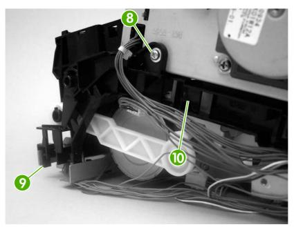
Figure 5-63 Remove the pickup-drive assembly (6 of 13)
