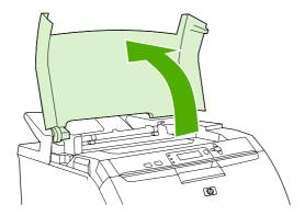
2. If the jammed sheet is visible, remove it and then close the upper cover.
