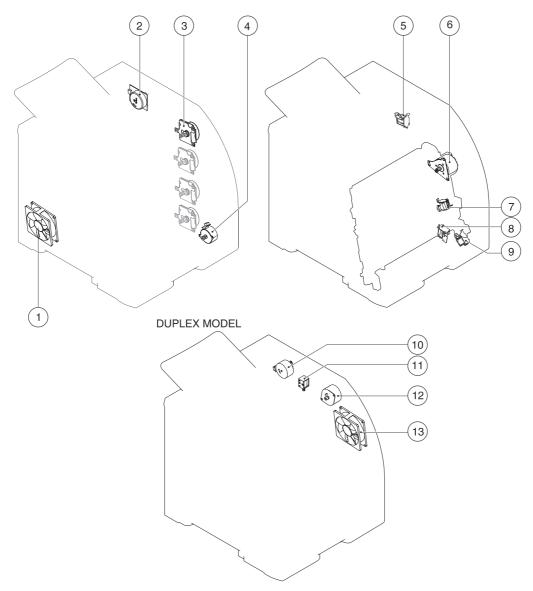
Figure 4-3 Motors, fans, and solenoids
