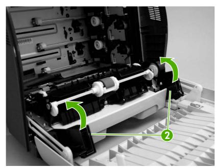
Figure 5-5 Remove the front cover (2 of 7)
