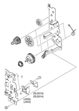
Figure 7-13 Developing separation-drive assembly
