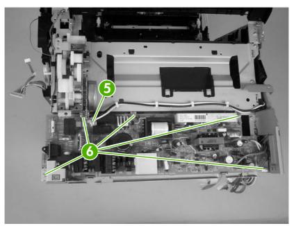
Figure 5-82 Remove the low-voltage power-supply PCA (4 of 6)
