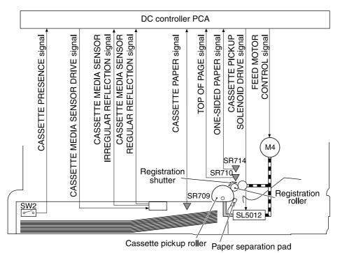
Figure 4-7 Cassette pickup mechanism
