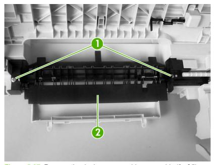
Figure 5-37 Remove the duplex-reverse-drive assembly (3 of 5)
