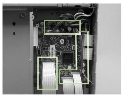
Figure 5-72 Remove the laser/scanner assembly (2 of 6)
