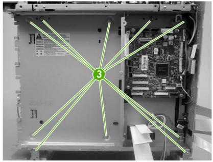
Figure 5-109 Remove the cartridge-sensor PCA (3 of 4)
