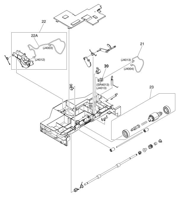
Figure 7-25 500-sheet feeder paper-pickup assembly
