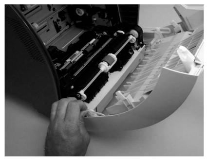
Figure 5-6 Remove the front cover (3 of 7)
