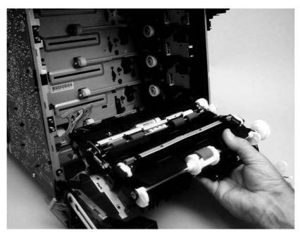
Figure 5-57 Remove the pickup-and-feed assembly (8 of 8)
