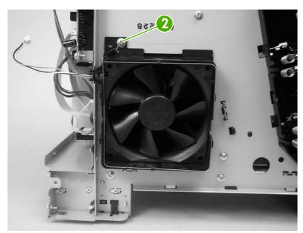
Figure 5-78 Remove the main fan (2 of 2)
