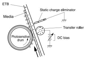
Figure 4-15 Separation from the drum
