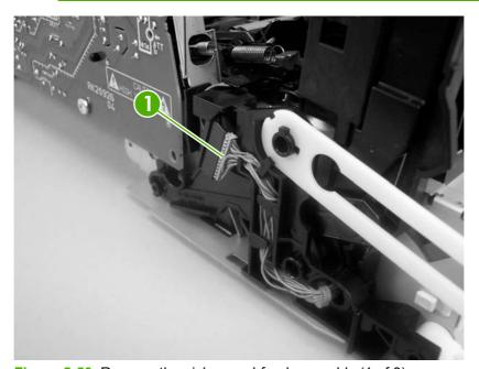
Figure 5-50 Remove the pickup-and-feed assembly (1 of 8)
