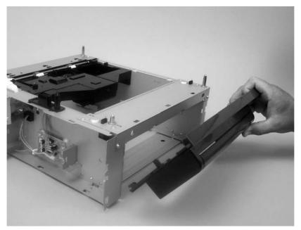
Figure 5-121 Remove the 500-sheet feeder rear cover (3 of 3)
