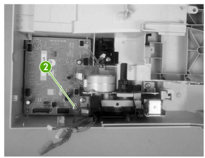
Figure 5-101 Remove the duplex-driver PCA (2 of 3)
