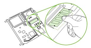
6. Push down on the DIMM until both latches engage the DIMM.
