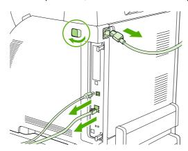
2. On the right side of the printer, gently pull the black tabs together, and then pull the formatter assembly from the printer.
