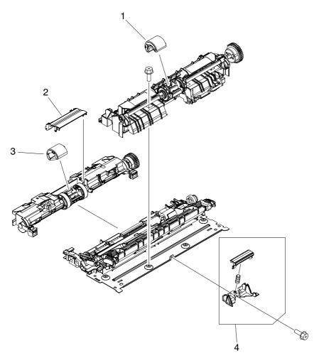
Figure 7-16 Paper-pickup assembly (HP CLJ 3600/3800)
