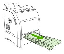
4. If the jammed sheet is visible, remove it.
