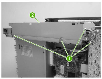
Figure 5-107 Remove the cartridge-sensor PCA (1 of 4)
