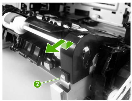
Figure 5-51 Remove the pickup-and-feed assembly (2 of 8)
