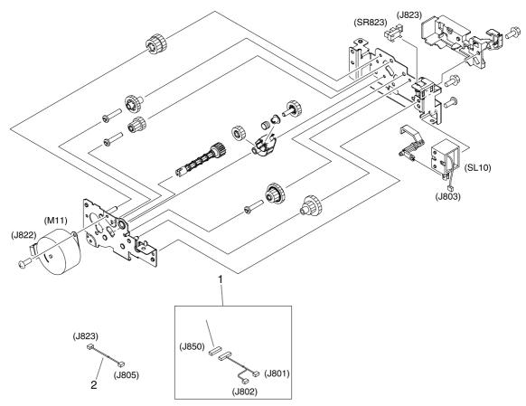
Figure 7-12 Duplexing reverse-drive assembly (duplex models)
