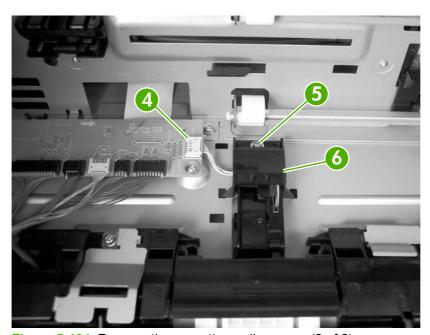
Figure 5-104 Remove the cassette media sensor (2 of 2)
