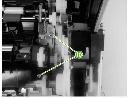
Figure 5-56 Remove the pickup-and-feed assembly (7 of 8)
