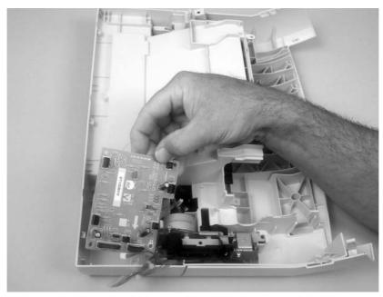
Figure 5-102 Remove the duplex-driver PCA (3 of 3)
