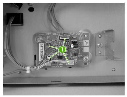
Figure 5-122 Remove the 500-sheet-feeder driver PCA (1 of 2)
