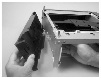
Figure 5-118 Remove the 500-sheet feeder left cover (5 of 5)
