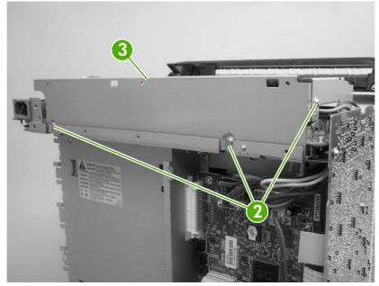
Figure 5-80 Remove the low-voltage power-supply PCA (2 of 6)
