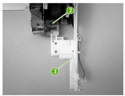
Figure 5-59 Remove the pickup-drive assembly (2 of 13)
