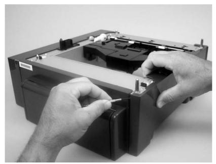
Figure 5-117 Remove the 500-sheet feeder left cover (4 of 5)
