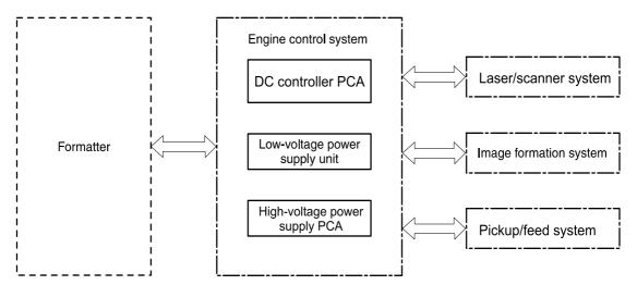
Figure 4-1 Engine control system components
