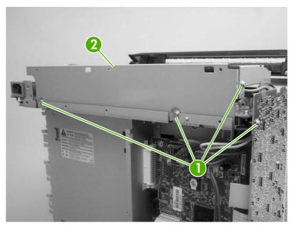
Figure 5-71 Remove the laser/scanner assembly (1 of 6)
