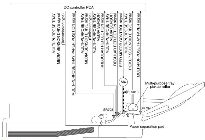
Figure 4-8 Multipurpose-tray pickup mechanism
