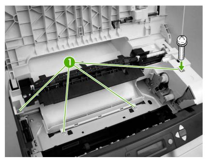
Figure 5-13 Remove the upper cover (3 of 5)
