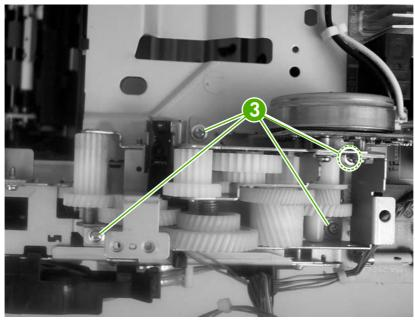
Figure 5-43 Remove the fuser drive assembly (2 of 4)
