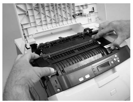
Figure 5-30 Remove the fuser
