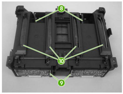
Figure 5-76 Remove the laser/scanner assembly (6 of 6)
