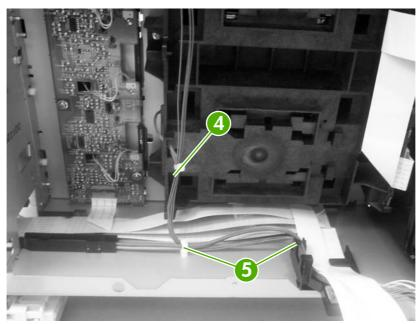
Figure 5-74 Remove the laser/scanner assembly (4 of 6)
