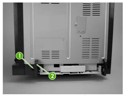
Figure 5-17 Remove the rear lower cover (2 of 2)
