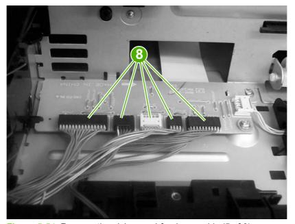
Figure 5-54 Remove the pickup-and-feed assembly (5 of 8)
