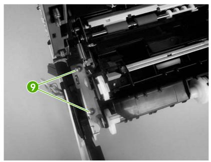
Figure 5-55 Remove the pickup-and-feed assembly (6 of 8)
