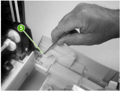
Figure 5-8 Remove the front cover (5 of 7)
