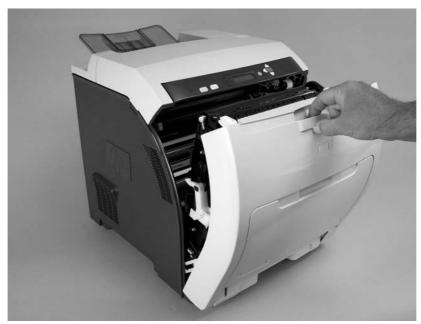
Figure 5-2 Remove the print cartridges (1 of 2)
