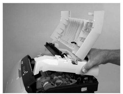
Figure 5-15 Remove the upper cover (5 of 5)
