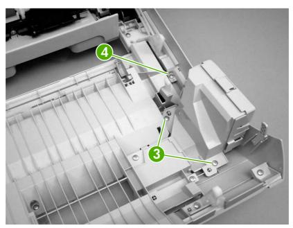
Figure 5-7 Remove the front cover (4 of 7)
