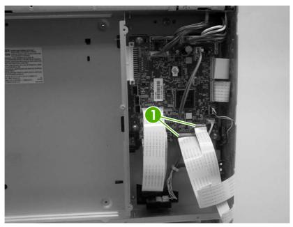
Figure 5-88 Remove the high-voltage power supply (1 of 3)
