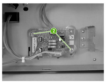
Figure 5-123 Remove the 500-sheet-feeder driver PCA (2 of 2)
