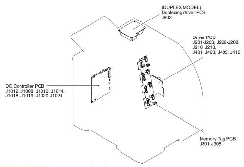
Figure 6-5 Printer connector locations
