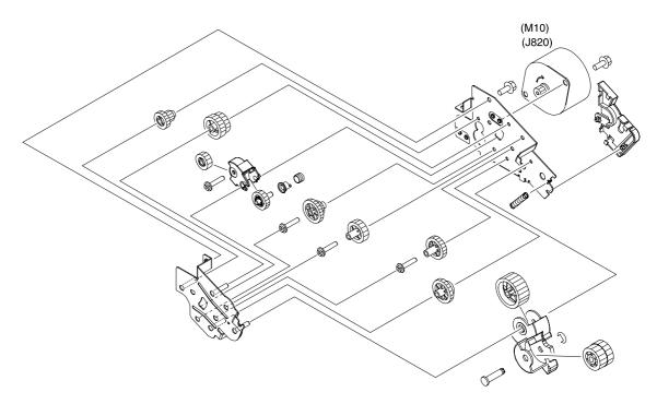
Figure 7-11 Duplexing-feed drive assembly (duplex models)
