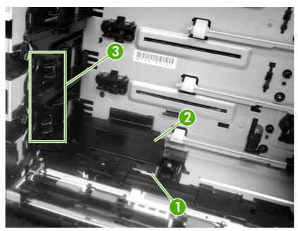
Figure 5-97 Remove the pickup-and-feed driver PCA (1 of 3)
