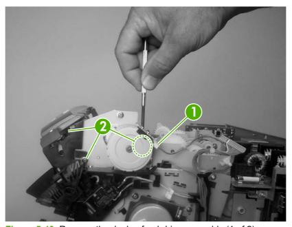
Figure 5-40 Remove the duplex-feed-drive assembly (1 of 2)
