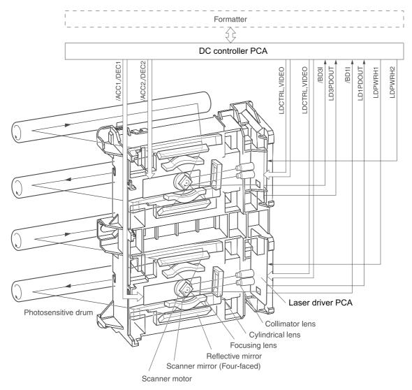
Figure 4-4 Laser/scanner system
