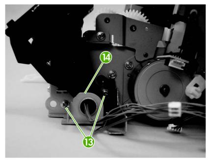
Figure 5-66 Remove the pickup-drive assembly (9 of 13)
