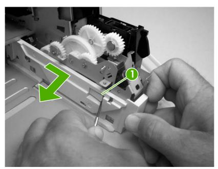
Figure 5-58 Remove the pickup-drive assembly (1 of 13)
