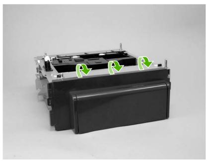
Figure 5-120 Remove the 500-sheet feeder rear cover (2 of 3)
