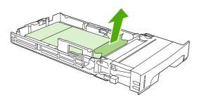
5. If the sheet is not visible, check inside the printer at the top of the tray opening. Remove any jammed media.
