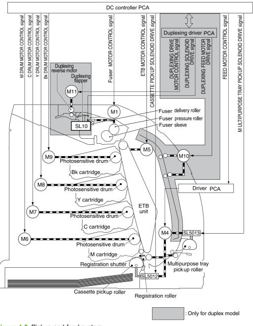
Figure 4-5 Pickup-and-feed system
