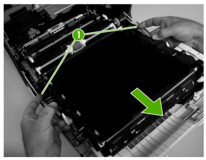
Figure 5-29 Remove the front ETB
