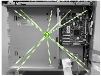
Figure 5-73 Remove the laser/scanner assembly (3 of 6)
