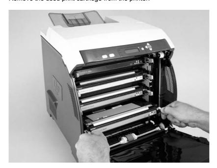
**3.** Remove the new print cartridge from the bag, and remove the tape-seal. Place the used print cartridge in the bag for recycling.
