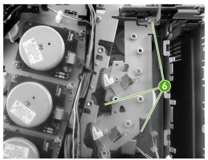
Figure 5-49 Remove the developing separation-drive assembly (4 of 4)
