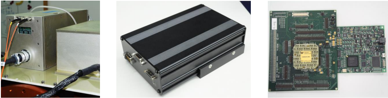
Figure 29. The three electronics packages used to test detectors are shown here. Electronics from left to right: Astronomical Research Camera Controller; JMClarke Engineering, Teledyne SIDECAR ASIC.
