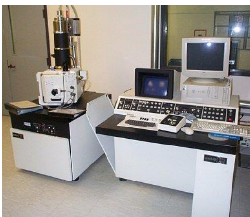
Figure 34. (left) The Amray 1830 Scanning Electron Microscope is used to image devices. On the right, a SEM image of a device that has been prepared for indium bump deposition.
