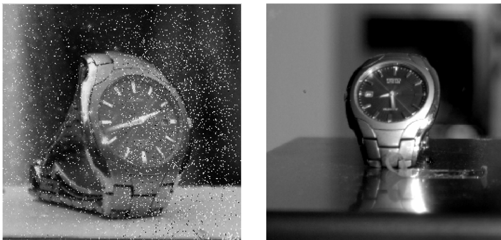
Figure 6. The picture on the left was taken with a previous version of the photon counting imaging detector, whereas the one on the right was taken with the most recent version of the detector. The images were taken under similar conditions. The images have had minimal processing performed on them and the image quality is significantly improved with the newest device.
