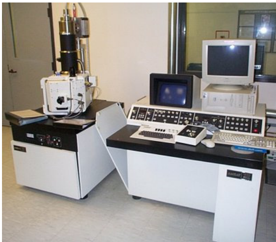
Figure 22. (left) The Amray 1830 Scanning Electron Microscope is used to image devices. (right) SEM image of a device that has been prepared for indium bump deposition.
