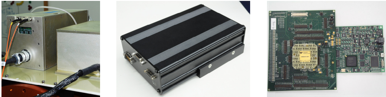
Figure 18. The three electronics packages used to test detectors. Electronics from left to right: Astronomical Research Camera Controller; JMClarke Engineering, Teledyne SIDECAR ASIC.
