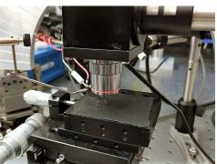
Figure 53. The electroluminescence measurement setup includes a rotating testing stage (right) and a FLAME 200 nm - 850 nm spectrometer (left).
