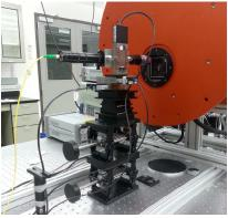
Figure 49. In the photo above, a laser spot projector with a threeaxis motion control system projects a small spot of light within individual pixels of detectors in order to measure the response in all regions of a pixel.
