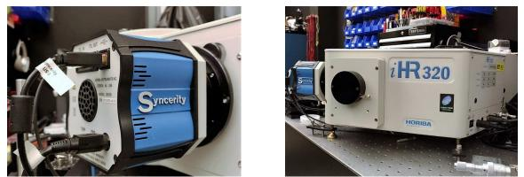
Figure 52. The Syncerity CCD Array detector (left) and the HR320 spectrometer (right) are part of the photoluminescence system.
