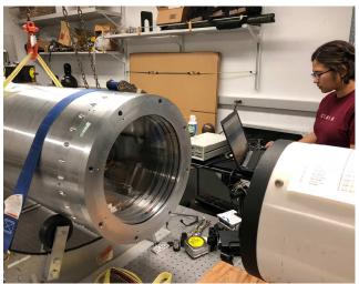
*Figure 16. Chi Nguyen takes test images to characterize the CIBER-2 telescope as the payload is being cooled to 77 K.*
