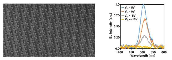
*Figure 28. (left) The picture above is a Nanowire LED array for high-resolution displays. (right) This picture demonstrates an individual sub-pixel control.*
