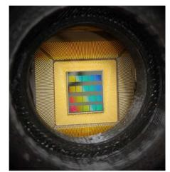
*Figure 26. This picture shows twenty 1 Mpixel QIS arrays residing in the detector housing.*
