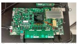
Figure 24. Above is the Xilinx VCU108 FPGA board that Davis used as the programmable system for communication between the user interface and peripheral QSFP modules.
