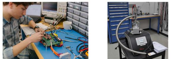
Figure 54. (left) Former CfD student, Ben Stewart is working with the FPGA-based control board, function generators, and oscilloscopes, used to develop CSTARS. (right) The picture shows one of the Oerlikon Leybold Turbolab turbo-molecular pumping stations in the lab.
