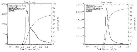
*Figure 6. This figure shows the dark current histograms for detectors F13 (left) and F17 (right) at 80 K.*
