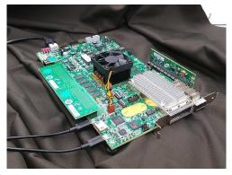
Figure 32. Shown above is the Xilinx FPGA used to create the PEK Evaluation Test Bed.
