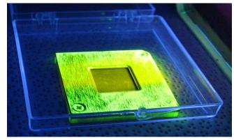
Figure 20. The yellow/green device above is a Quantum Dot coated detector in aluminum mask under UV illumination. The active area is 15 mm  $\times$  15 mm.
