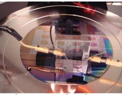
Figure 61. The image shows wafer testing using the probe station.
