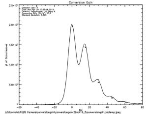
Figure 4. The graph shows the distribution of signal in the conversion gain analysis. The location of peaks corresponds to integer numbers of electrons detected as a signal. Location of peaks is determined from gaussian fitting and subtracting.
