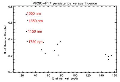
*Figure 7. This figure shows the persistence vs fluence plot for F17 at 1150, 1350, 1550, and 1750 nm.*
