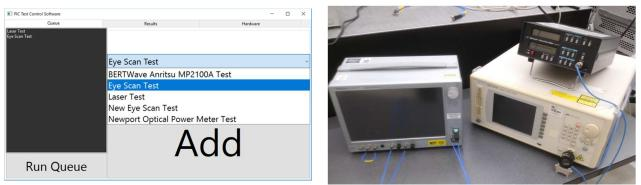
Figure 29. The left image shows the eye scan software that interacts with various measurement instruments, such as the set up shown on the right.
