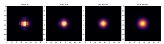
Figure 2. The snapshots illustrate how combining the mean of an increasing number of Gaussian source thumbnails improves the PSF via the stacking process. After combining sources, the PSF resembles that of the original point sources.
