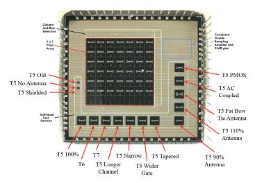
*Figure 19. Above is a photo of the generation II MOSIS THz device. Fifteen test structures are along the edges.*
