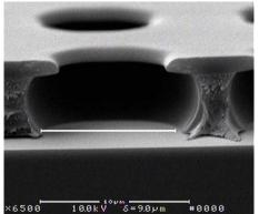
Figure 59. (left) CfD researchers use the Amray 1830 Scanning Electron Microscope to image devices. (right) The SEM image shows a sample prepared for indium bump deposition.
