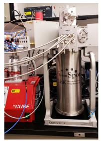
Figure 10. The Integrated Photonics Laboratory has a single photon detector system.
