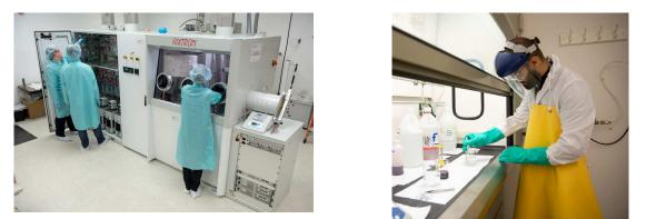
Figure 56. (left) PhD student Mohad Baboli loads a sample in the AIXTRON  $3 \times 2$  Close Coupled Showerhead metal-organic chemical vapor deposition reactor, part of the MOVPE. (right) PhD student Alireza Abrand is processing samples in the fume hood.
