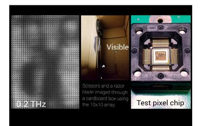
Figure 33. (left): A 0.2 THz mosaic image of the scissor and razor blade enclosed in a box as imaged by the 10x10 pixel array is shown. The pattern visible is due to variations of pixel response and will be accounted for using the power relation found from work with single pixel testing. (middle): You can see a visible image of the inside of the box. (right): Pictured here is a close up of one of the single pixel chips with varied designs.
