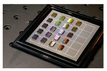
*Figure 38. The image above shows photonic chips designed by Stefan Preble's Integrated Photonics Group and AIM Photonics partners.*
