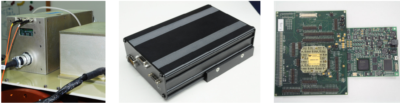
Figure 33. The three electronics packages used to test detectors are shown here. Electronics from left to right: Astronomical Research Camera Controller; JMClarke Engineering, Teledyne SIDECAR ASIC.
