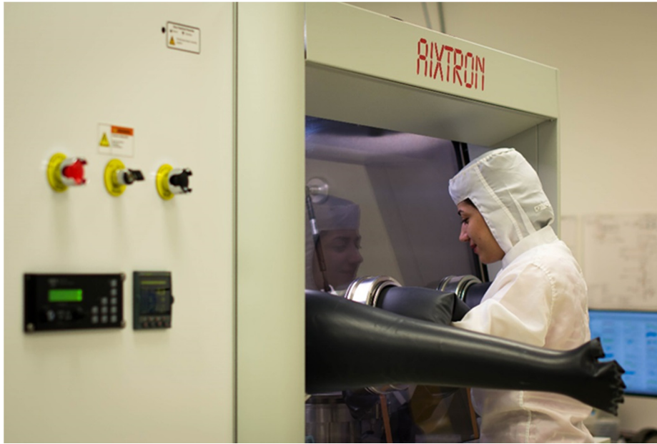
Figure 27. Mohad is seen here loading a sample in the AIXTRON 3×2 Close Coupled Showerhead metal-organic chemical vapor deposition (MOCVD; RIT NanoPower Research Laboratories) reactor for crystal growth of III-V semiconductor nanowires.
