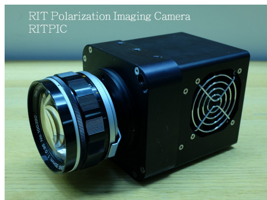
Figure 7. The RIT Polarization Imaging Camera is a compact, snapshot, imaging polarimeter, suitable for use with a wide range of imaging systems, from telescopes to microscopes. Here, RITPIC is shown with a f/0.95 photographic lens.
