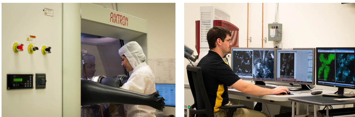
Figure 45. (left) Ph.D. student Mohad Baboli loads a sample in the AIXTRON 3x2 Close Coupled Showerhead metal-organic chemical vapor deposition reactor, part of the MOVPE. (right) Ph.D. student Thomas Wilhelm uses a TESCAN MIRA3 scanning electron microscope to analyze samples for use in metal-assisted chemical etching experiments.
