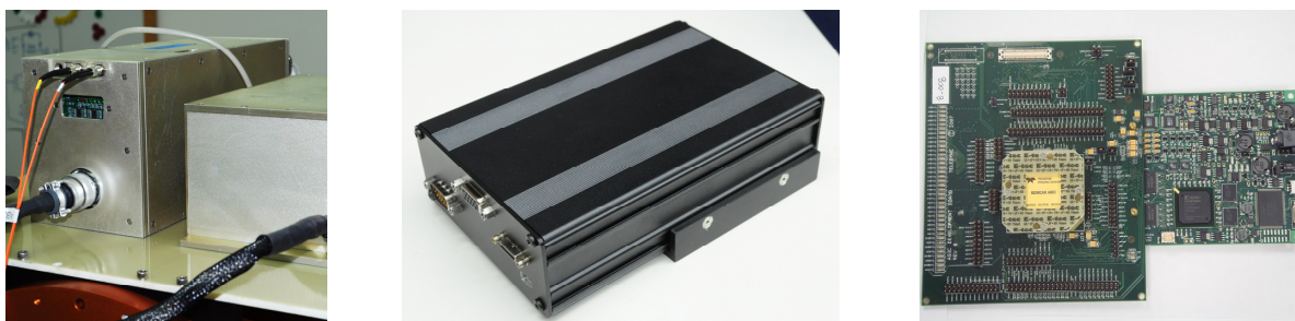
Figure 47 The three electronics packages used to test detectors are the Astronomical Research Camera Controller (left), JMClarke Engineering (middle), and the Teledyne SIDECAR ASIC (right).
