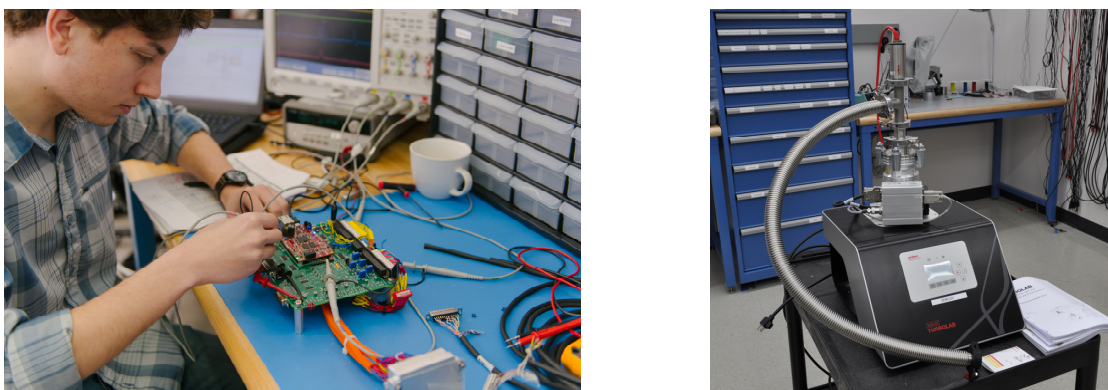
Figure 54. (left) Former CfD student, Ben Stewart is working with the FPGA-based control board, function generators, and oscilloscopes, used to develop CSTARS. (right) The picture shows one of the Oerlikon Leybold Turbolab turbo-molecular pumping stations in the lab.
