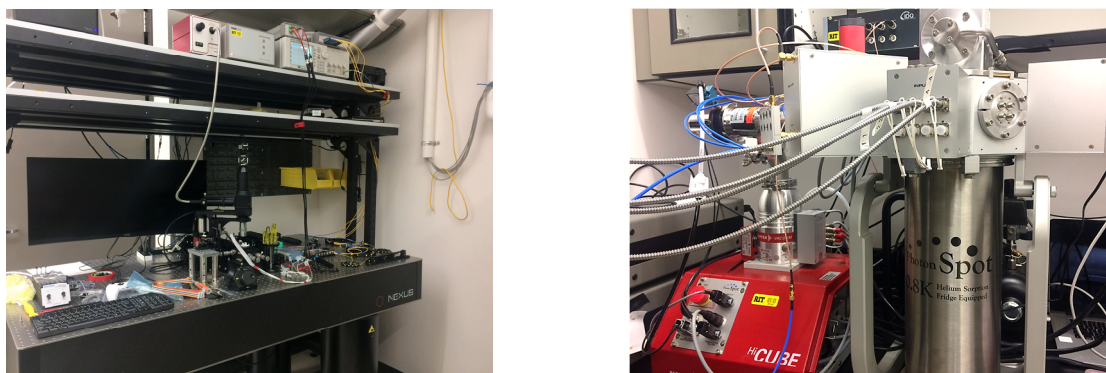
Figure 51. (left) The photo above shows the optical table used to run quantum integrated photonic experiments in the newly opened Integrated Photonics Lab. (right) This photo shows the Photon Spot single photon detector system funded by AFOSR.
