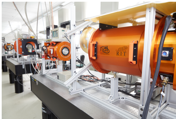
Figure 46. The photo above shows the cryogenic dewars in the Rochester Imaging Detector Laboratory.
