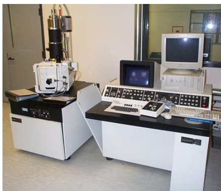
Figure 59. (left) CfD researchers use the Amray 1830 Scanning Electron Microscope to image devices. (right) The SEM image shows a sample prepared for indium bump deposition.
