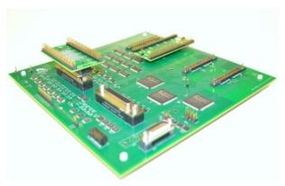
Figure 61. This image shows a cryogenic multi-layer circuit board designed in the CfD and populated in CEMA. All of the components on this board work at temperatures as low as 40 K, nanoTorr pressure levels, and in the presence of high energy particle radiation.
