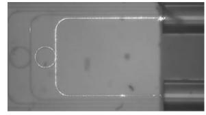
Figure 6. The image above shows a ring resonator operating at UV wavelengths. The photo is curtesy of Michael Fanto, RIT and AFRL.
