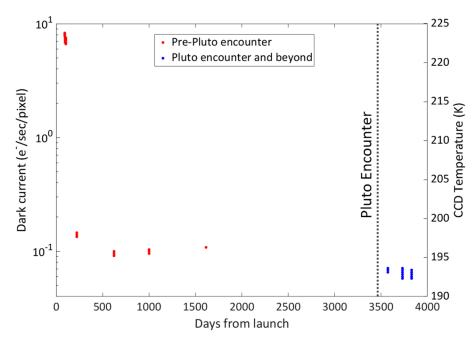
Figure 1. As expected, dark current and CCD temperature continue to decrease with increasing mission time and distance from the Sun during the New Horizons' space mission. The error in the LORRI images due to dark current becomes more negligible compared to other sources.
