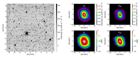
Figure 2. (left) Here is an example of an image taken by LORRI. (right) The graphs show comparisons of a PSF made by stacking stars in that image together  $(P_S)$  versus a final deconvolved reconstructed PSF  $(P_{IBP})$  in both linear (top row) and logarithmic (bottom row) scales.
