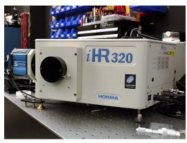
Figure 50. The Syncerity CCD Array detector (left) and the iHR320 spectrometer (right) are part of the photoluminescence system.
