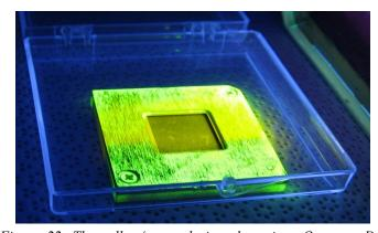
Figure 22. The yellow/green device above is a Quantum Dot coated detector in an aluminum mask under UV illumination. The active area is 15 mm $\times$ 15 mm.
