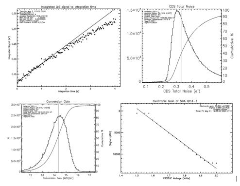
Figure 4. (top left) This figure shows room temperature results for the QISPF. A linear fit gives dark of 0.03 e<sup>-</sup>/s/pix. (top right) The average total noise of the detector array is 0.34 e<sup>-</sup>. (bottom left) The average conversion gain of the detector array is 14.4 ADU/e<sup>-</sup>. (bottom right) The electronic gain of a pixel is 36.0  $\mu$ V/e<sup>-</sup>which is estimated through a linear fit to the digitized reset signal as a function of reset voltage.
