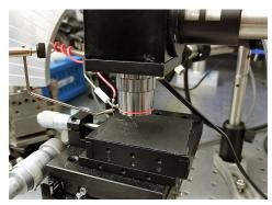
Figure 57. The electroluminescence measurement setup includes a rotating testing stage (right) and a Flame 200 nm – 850 nm spectrometer (left).
