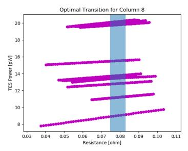
Figure 17. This figure shows the testing of advanced detector biasing technique. The shaded region shows the optimal electrical resistance needed to keep the most detectors operating. This is done per column since detectors are electrically coupled in this configuration. These values are from static lab data taken at room temperature, and will change due to change in atmospheric conditions and the source being observed.
