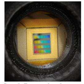
Figure 3. The image above shows twenty megapixel QIS arrays residing in the detector housing. Each detector has a side length of 1.1  $\mu$ m. All twenty detectors fit within a square millimeter.
