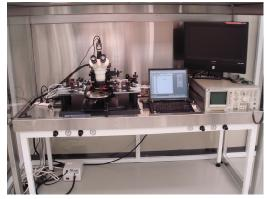
Figure 58. Shown above is the flow-bench lab probe station CfD researchers use to test device wafers.
