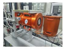
Figure 47. The four custom dewar test systems evaluate detectors in RIDL.
